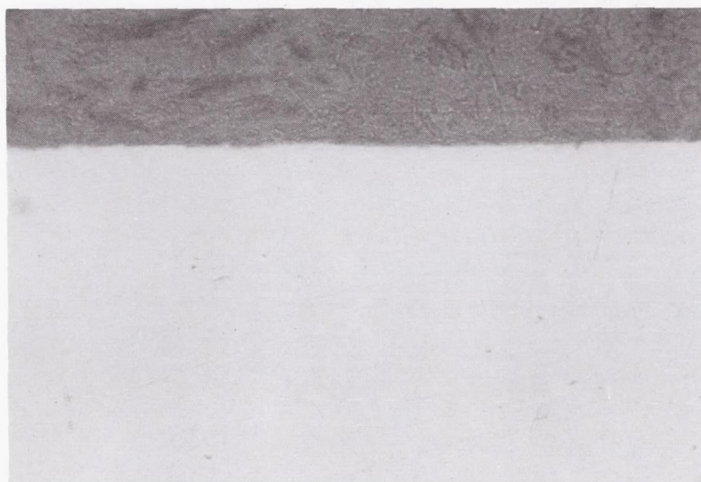
(a) Unnotched Specimen, Titanium 6Al-4V (200X)
