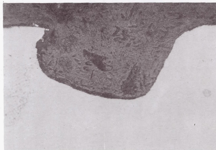
(b) Notched Specimen, Titanium 6Al-4V (200X)
