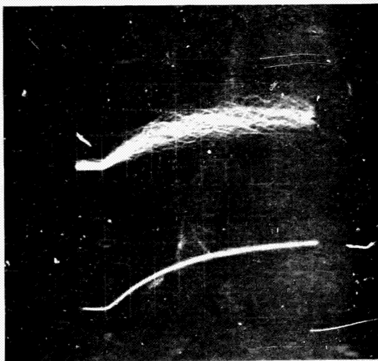
FIGURE D-7 INTEGRATOR OUTPUT OCEAN RETURN N_o/N_r = 10 DB SINE WAVE SIGNAL (TOP) S/N_r = 16 DB (BOT) AGC OPERATING DETECTOR BIASED 50 PULSES 0.1 V/CM 400 N SEC/CM
