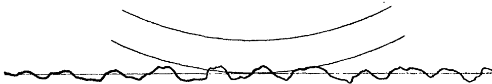
ILLUSTRATION OF REAL OCEAN AS A RADAR SCATTERING CROSS SECTION GENERATOR FIGURE A-10
