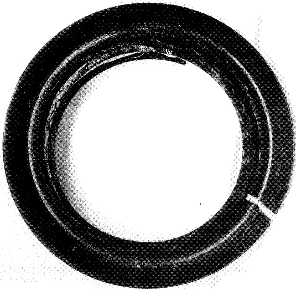
Figure 1. 45° V-Seal, 1300 Hours of Operation (No. 1 Seal - Inboard)
