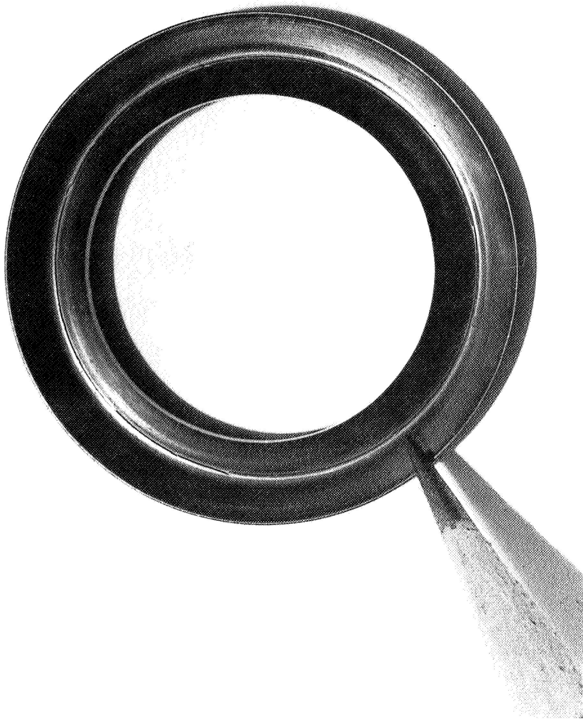
Figure 44. 45° V-Seal (Design A) Outboard Element after 13, 248, 747 Cycles
