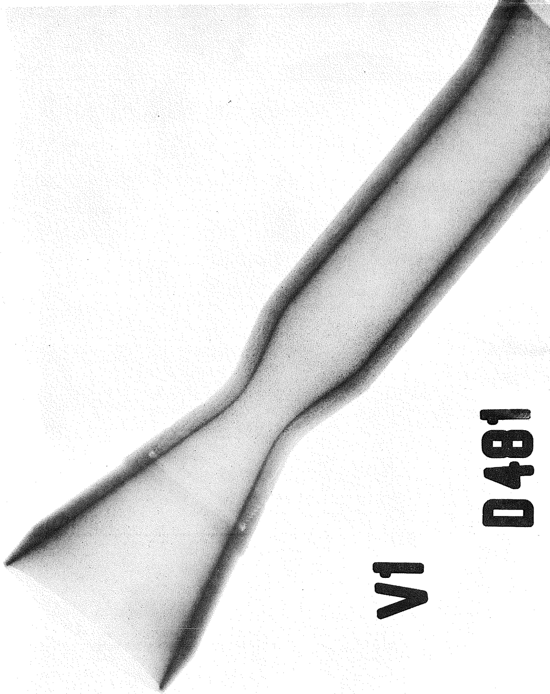
FIGURE 42. X-Ray Photograph of PG/Carbitex Thrust Chamber with RPG Nozzle Extension
