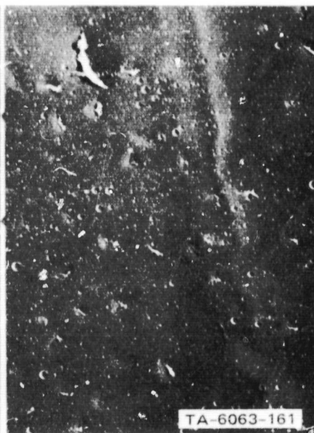
FIGURE 18 STEREO ELECTRON MICROGRAPH OF SPECIMEN 34 (Group IV) AFTER THERMAL CYCLING
