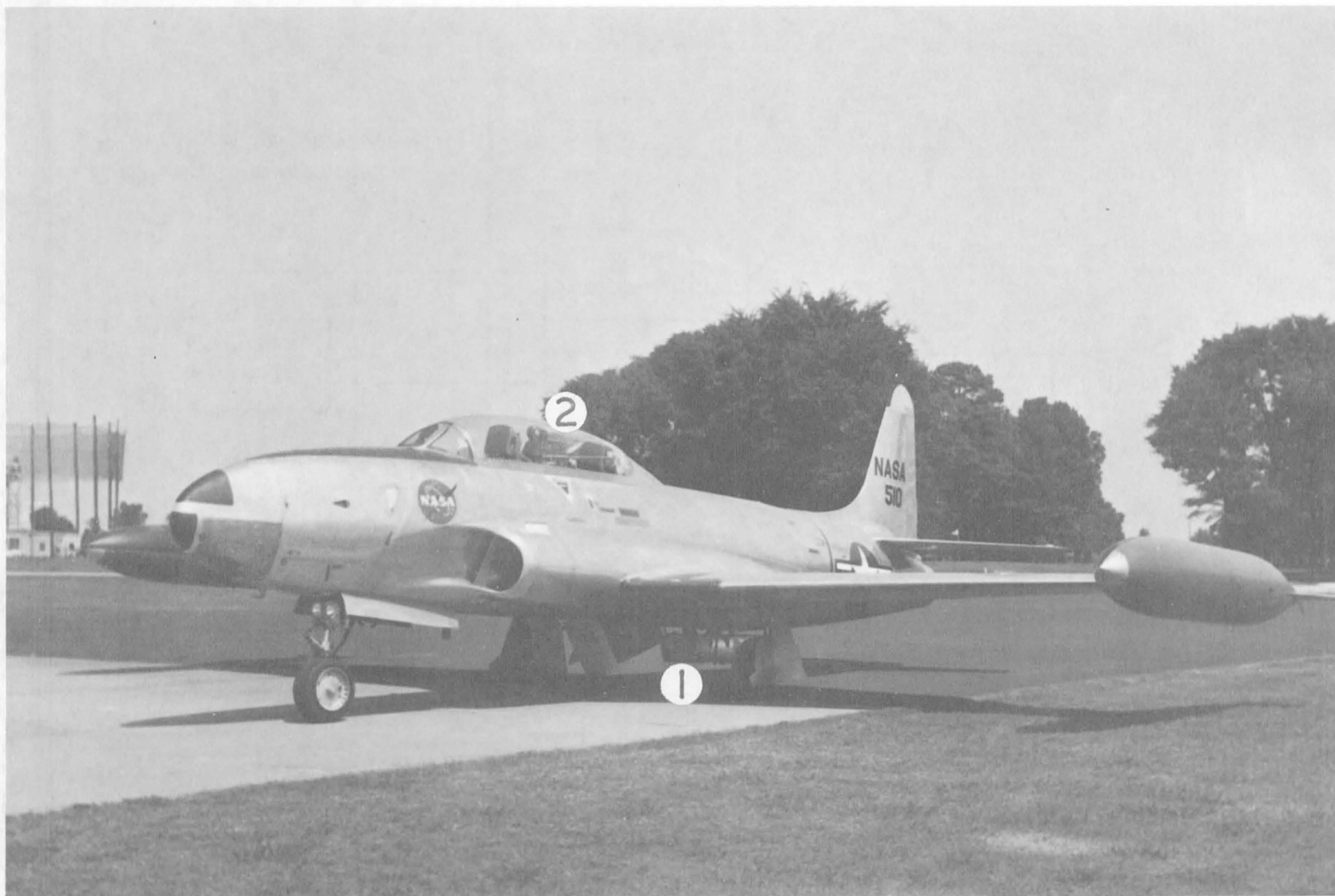
Figure 4.- The laser system installed in a T-33 jet airplane with the location of the equipment noted as ① transmitter and receiver subsystems and ② display and recording subsystem and the system controls.
