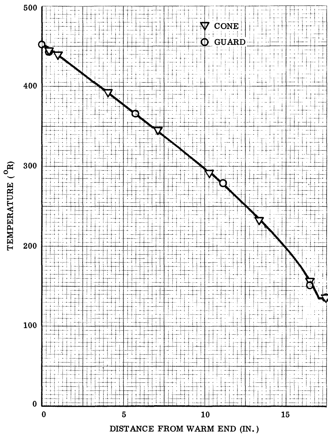
Fig. 58 Temperature Profile in Conical Support – Test V-1
