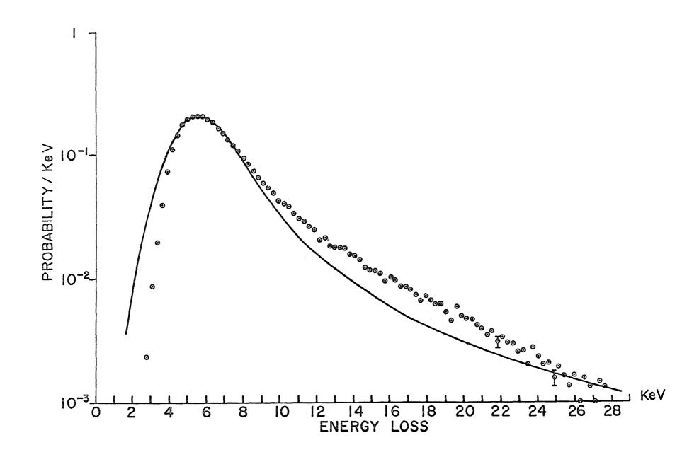
Frequency distribution of energy losses by protons of 46.4 MeV energy in a pathlength of  $1.33 \times 10^{-3}$  g/cm<sup>2</sup>.
