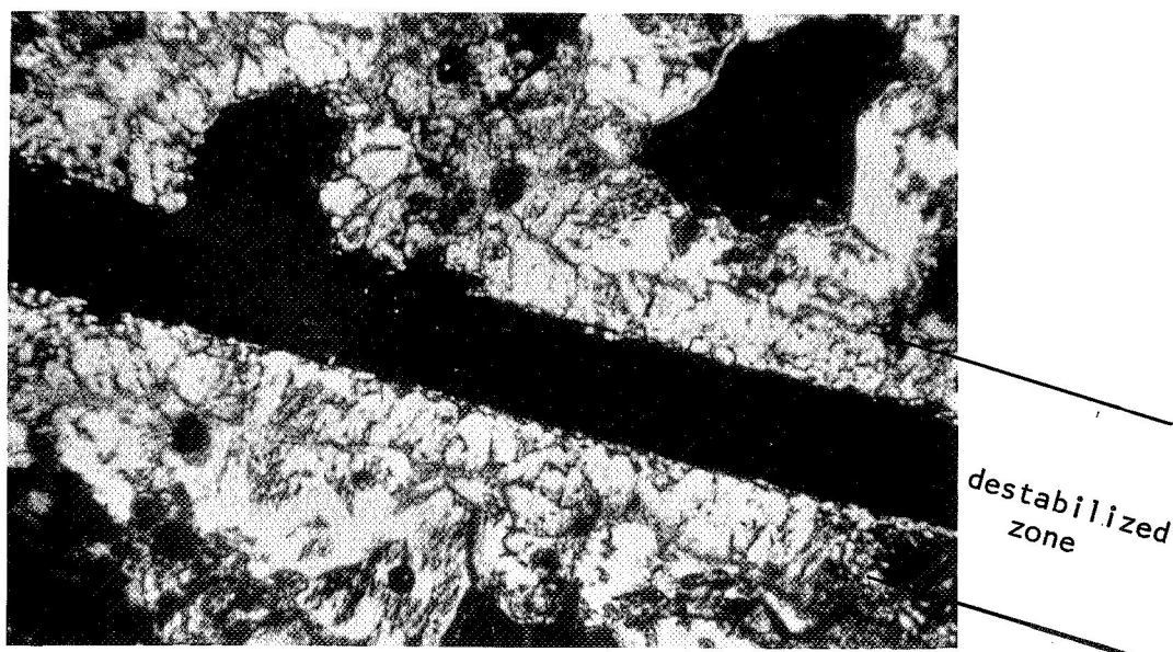
Figure 46. Cross-section of intermediate zone Type A material, F410 + 5v/o of 3.5 mil wire, propellant oxidation specimen, after 200 seconds exposure at 4200°F; transmitted polarized light, 150X.
