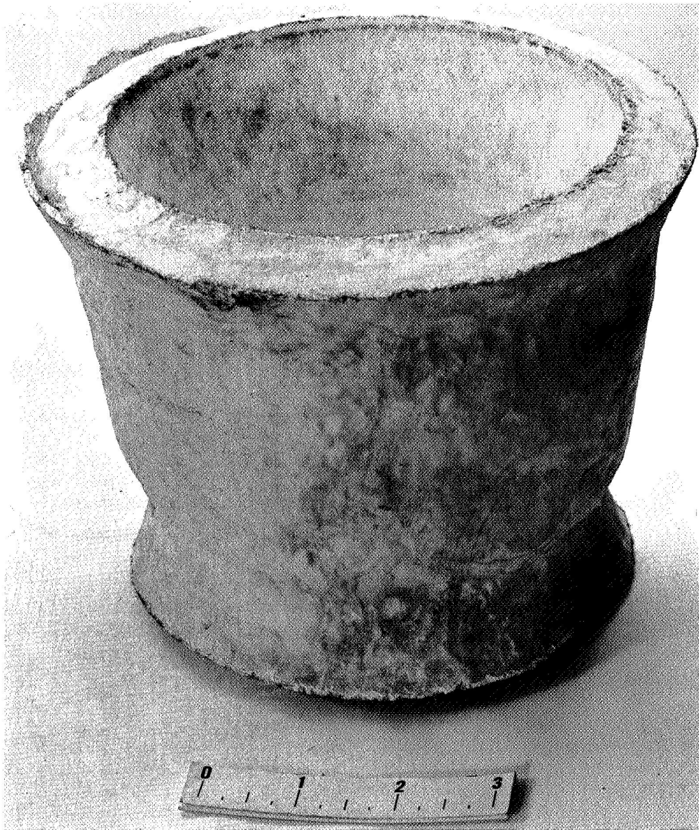
Figure 56. Isopressed billet of Type C material used in fabricating the 3 inch I.D. throat insert.
