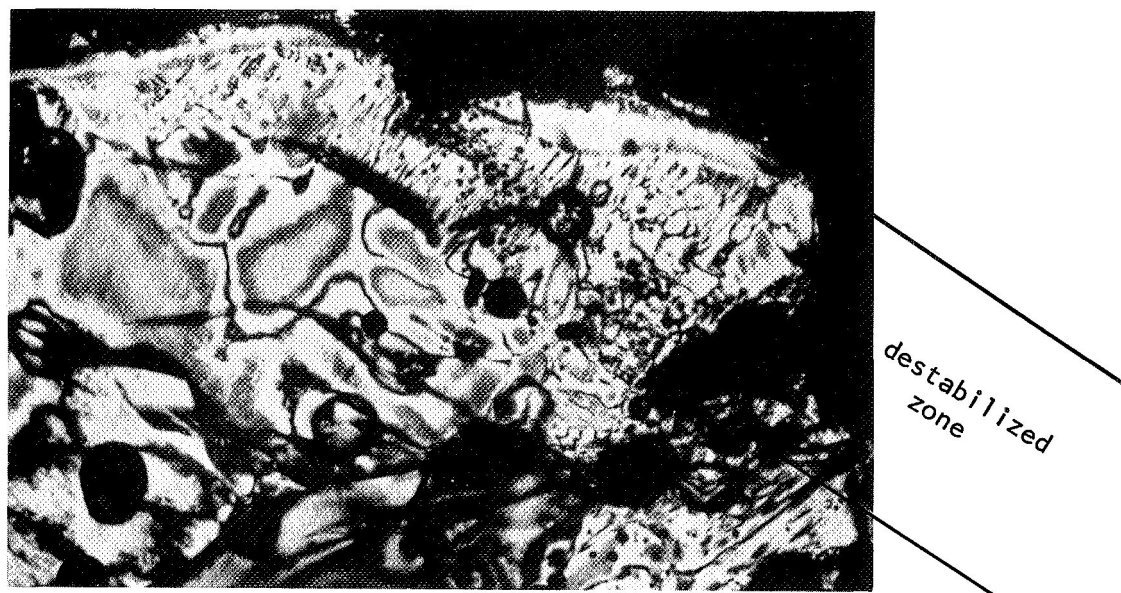
Figure 45. Cross-section of hot face of Type A material, F410 + 5v/o of 3.5 mil wire, propellant oxidation specimen after 200 seconds exposure at 4200°F. Transmitted polarized light, 370X.
