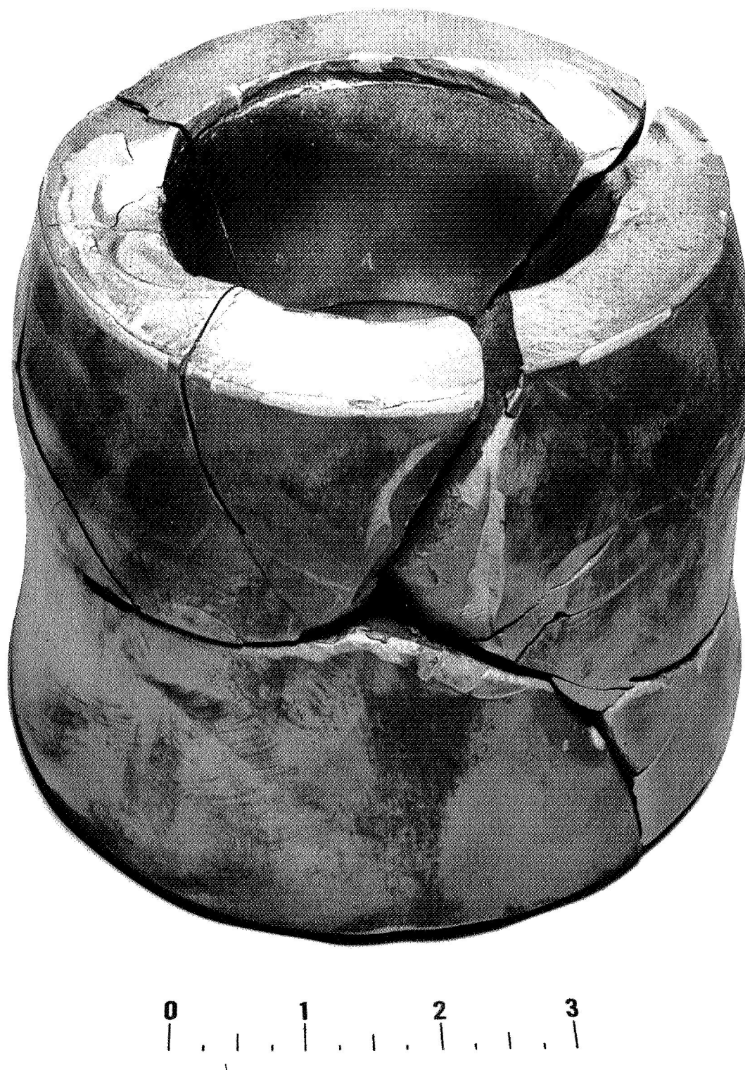
Figure 60. As-sintered unreinforced zirconia insert showing effects of the 167°F/hr heating rate during the sintering cycle.
