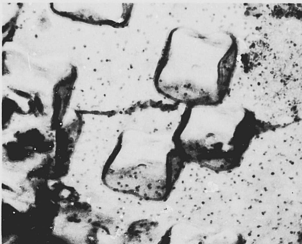
(a) Corrosion patterns on Al-4Cu (100000X)
