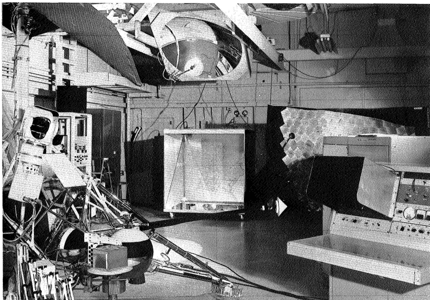
Fig. 1. Test facility with full-scale model spacecraft under collimated light source and, directly below light, 45-deg mirror for sun angles below 7 deg
