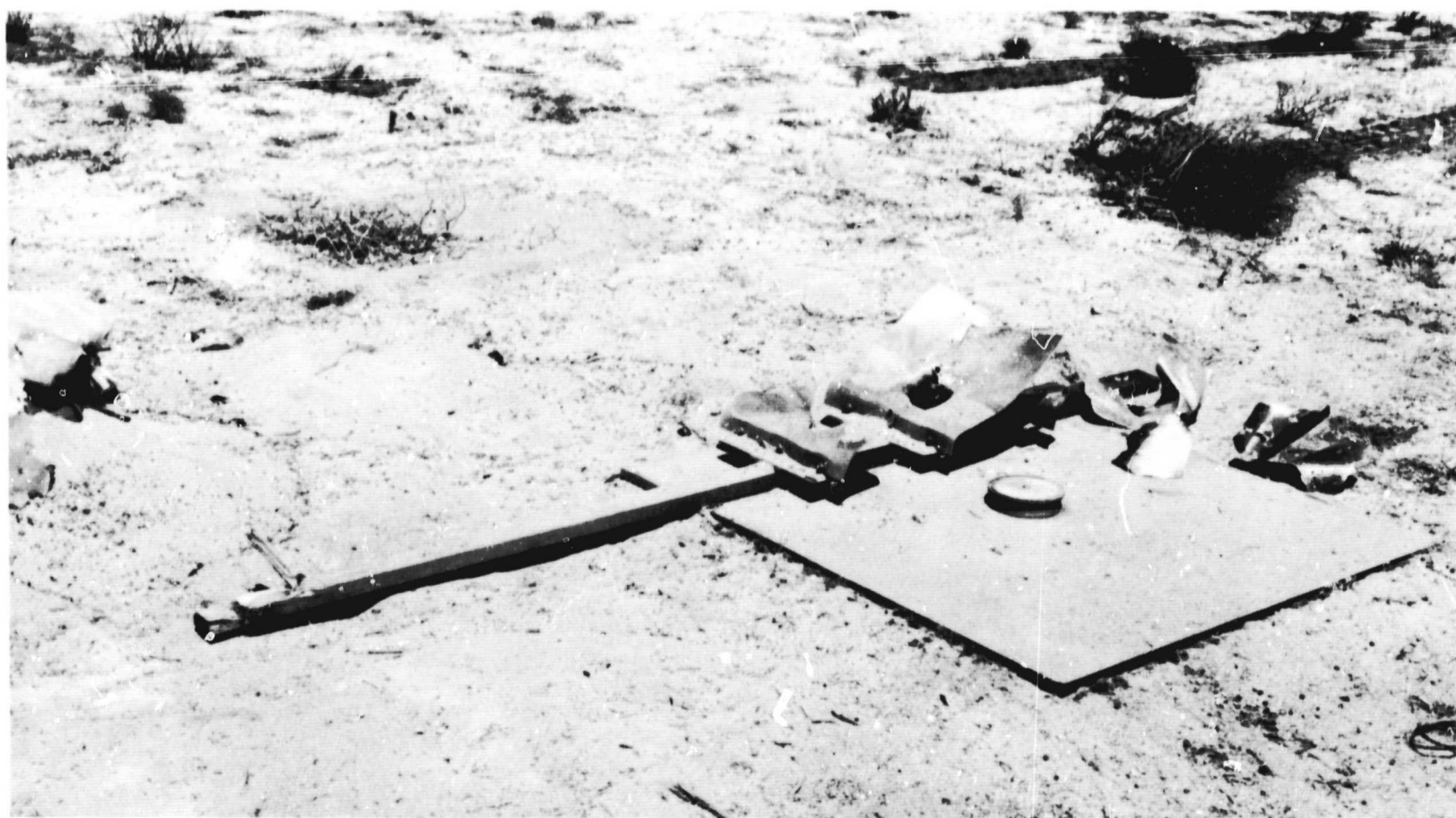
Fig. 6. Condition of plates after shaped-charge detonation
