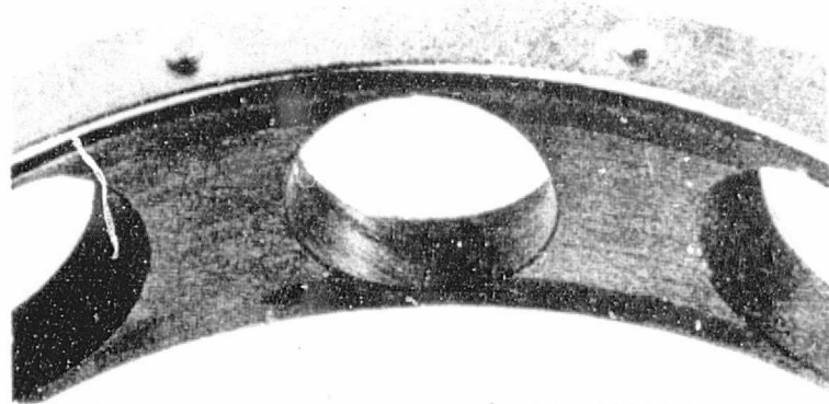
(b) GLASS-FIBER-FILLED PTFE (BEARING 15-S). CRACKS IN BALL POCKET AFTER 464 MINUTES.
