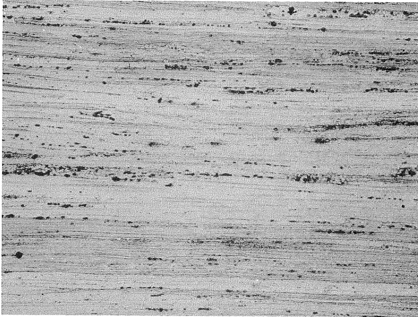
Fig. IV-5 Microstructure of Parent-Metal 7075-T6; Longitudinal Direction (Enlarged 100X)
