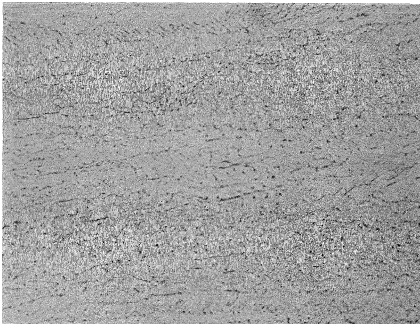
Fig. IV-10 Microstructure of Aged, Cryogenically-Stretched Type 301 Stainless Steel; Welded Metal; Longitudinal Direction (Enlarged 250X)
