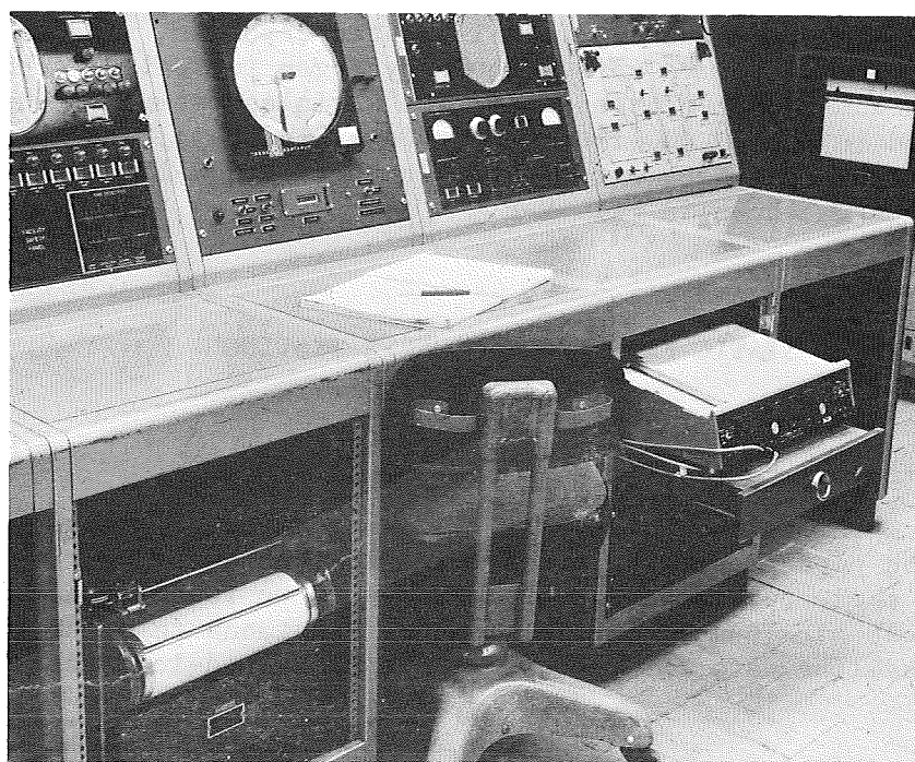
Fig. V-4 SRA-7 Recorder and X-Y Plotter Used with 400,000-lb Testing Machine
