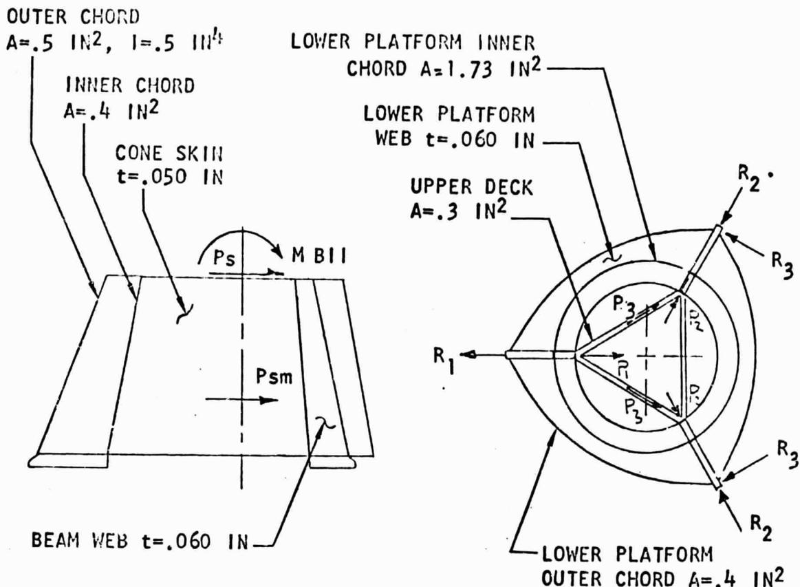
A. LOWER PLATFORM AND OUTER CHORD BENDING ENERGY
