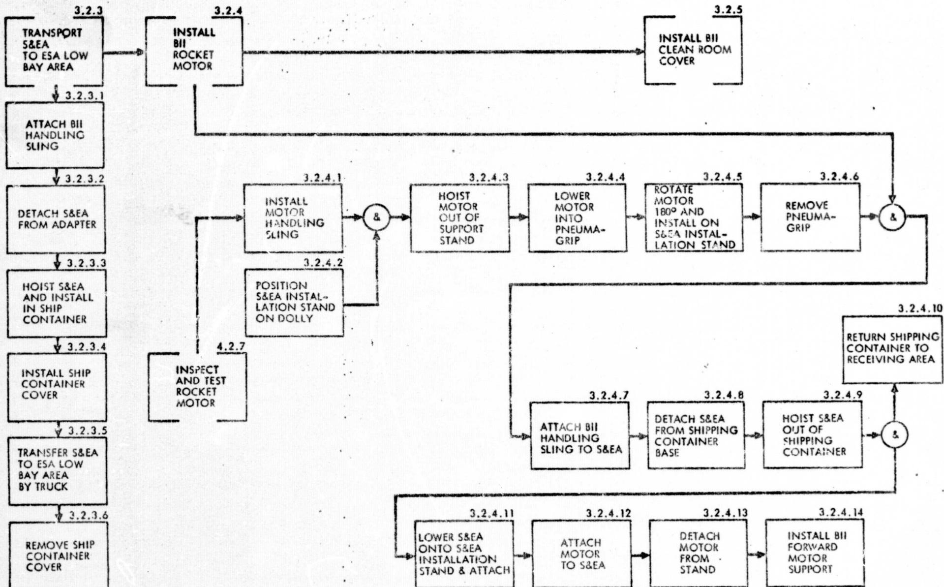
FIGURE 2.7-9: FUNCTIONAL FLOW 3.2.3 AND 3.2.4, TRANSPORT S&EA AND INSTALL ROCKET MOTOR
