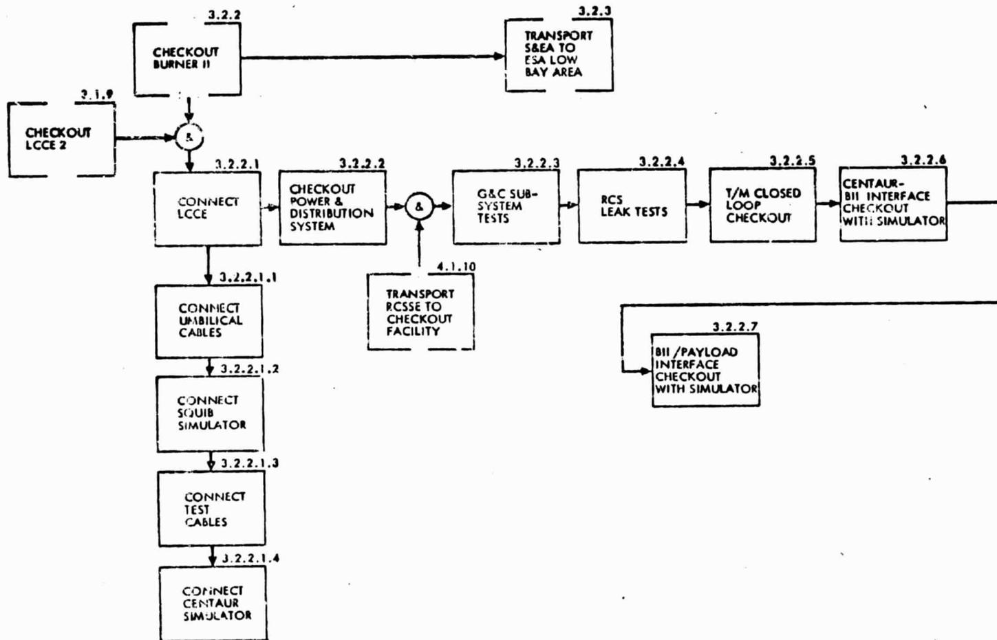
FIGURE 2. 7-8: FUNCTIONAL FLOW 3.2.3, CHECKOUT BURNER II
