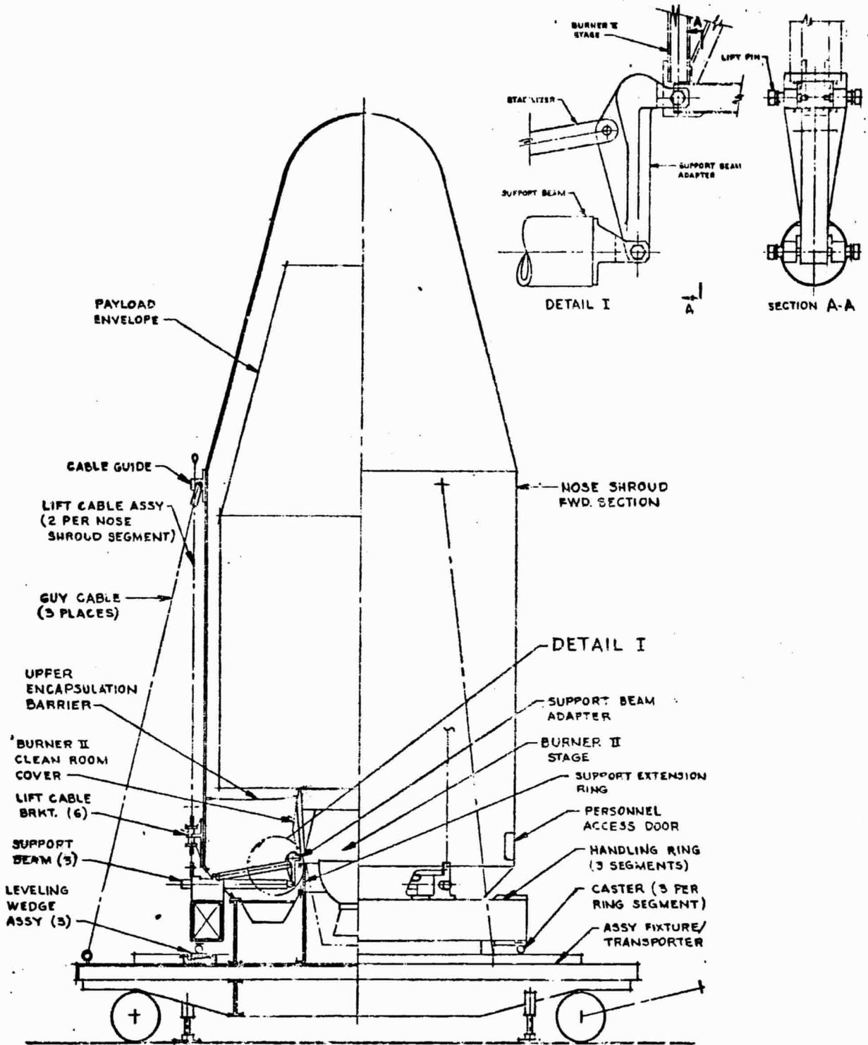
PAYLOAD/BURNER II ENCAPSULATION CONCEPT
