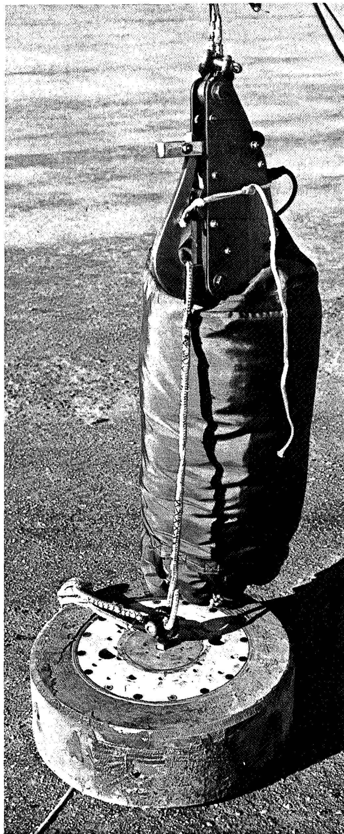
Fig. 4. Parachute pack for gliding test
