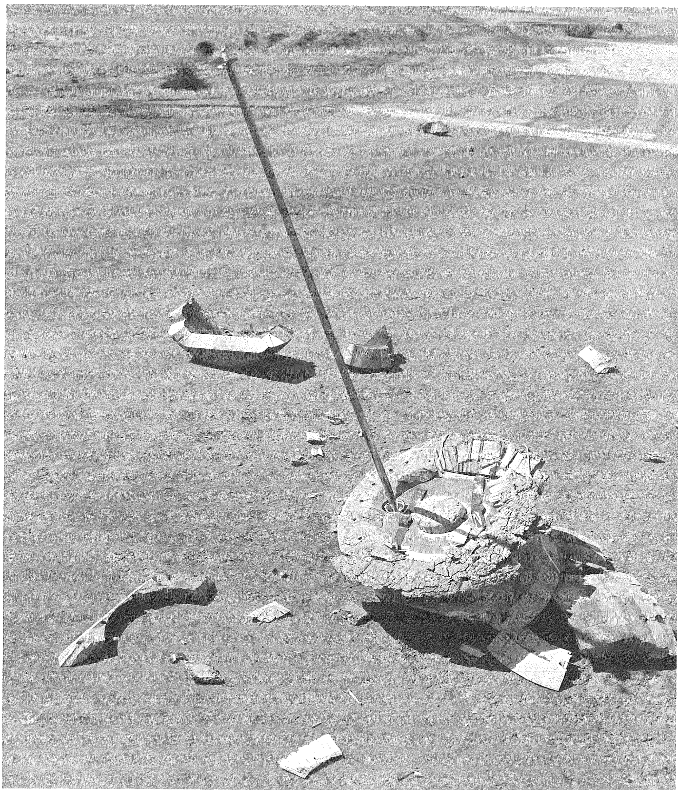
Fig. 5. Lander after drop on asphalt (nonyielding surface)
