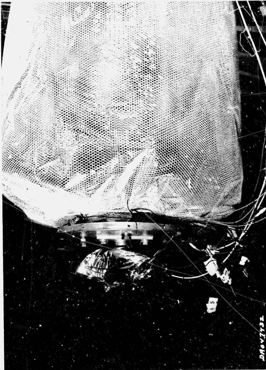
Figure IV-8 Composite Material Thermal Conductivity Specimen After Insulation
