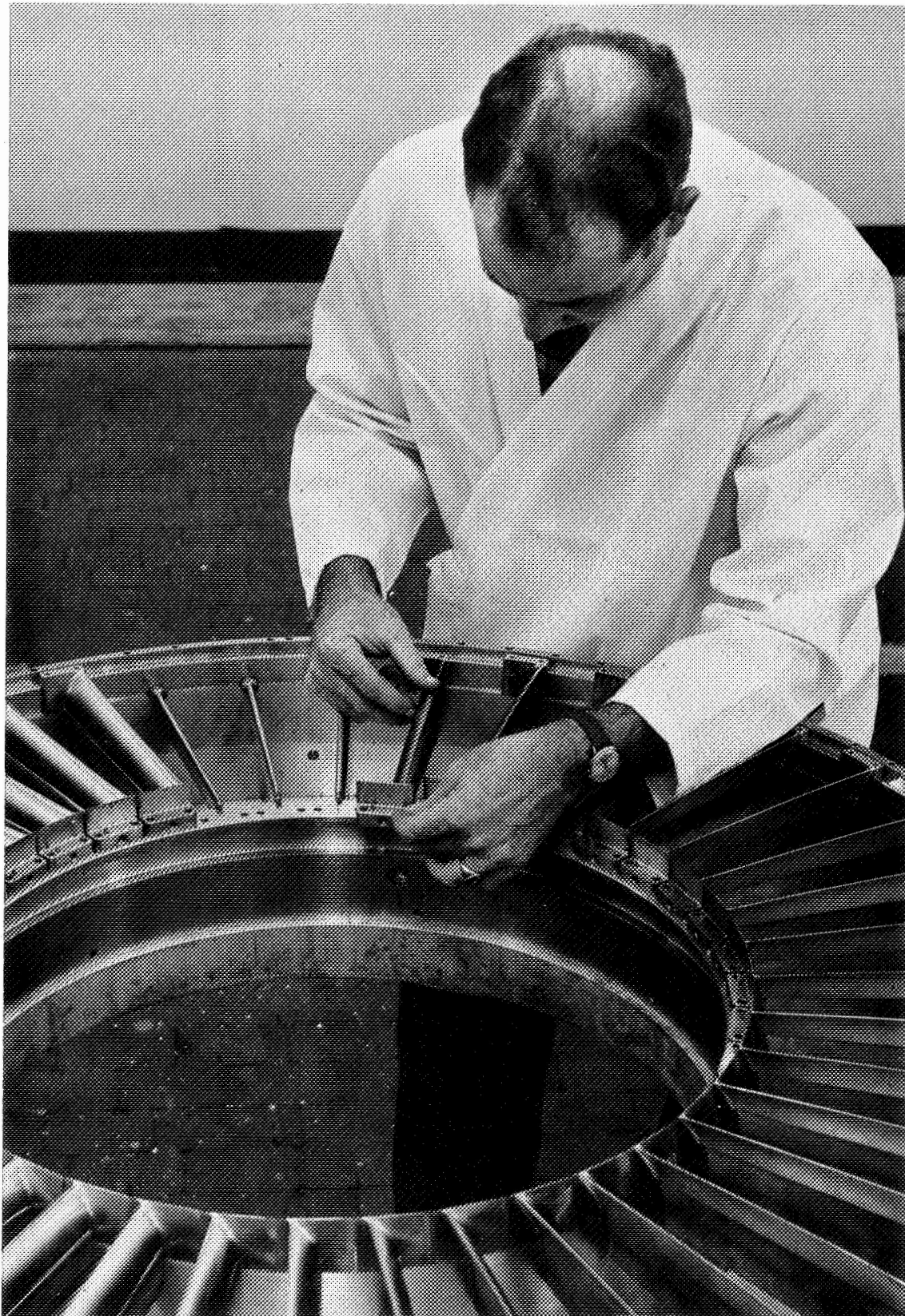
Figure 16. Variable Geometry Stator A Assembly
