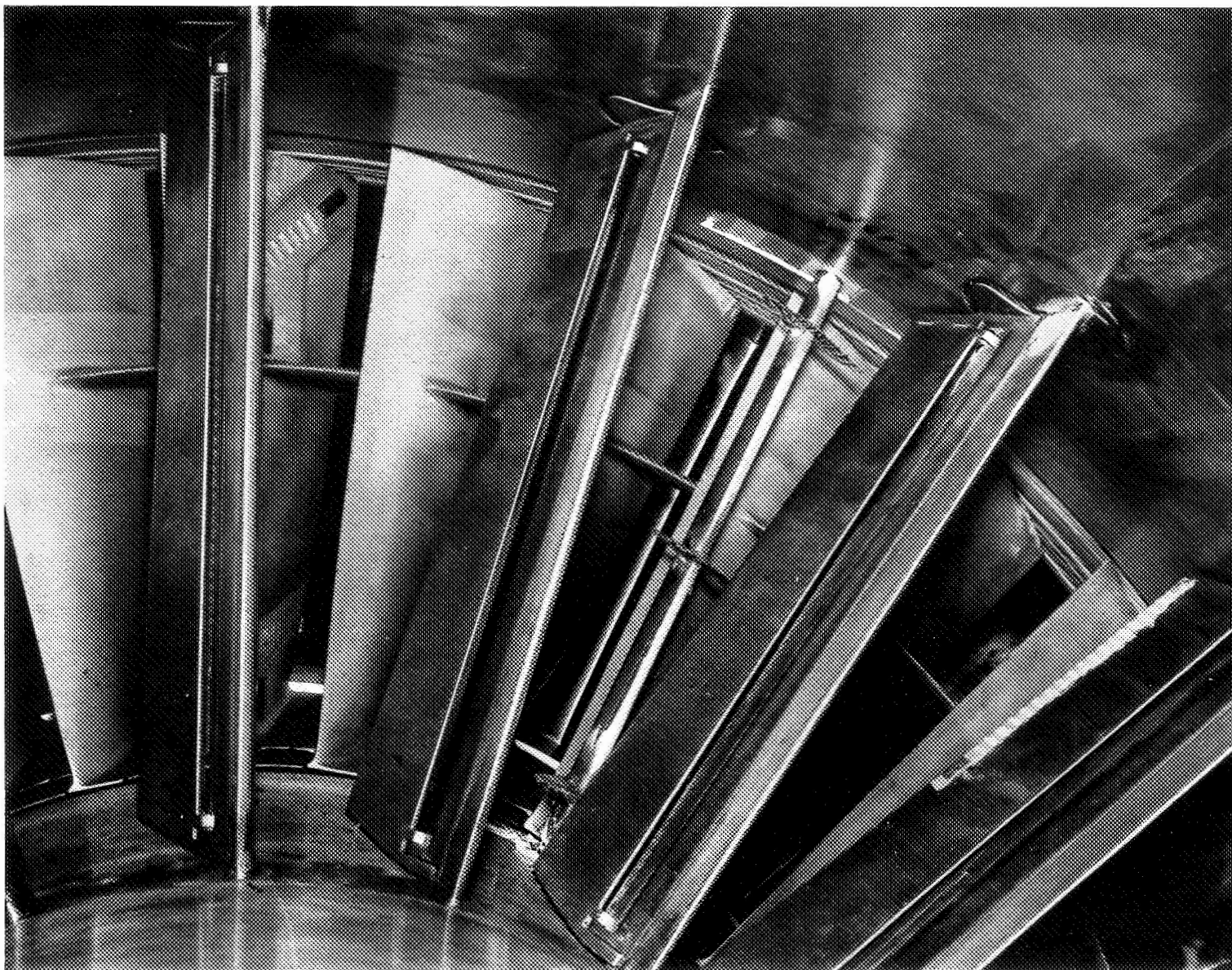
37 Figure 12. Variable Camber Inlet Guide Vane Assembly in SLTO Configuration
