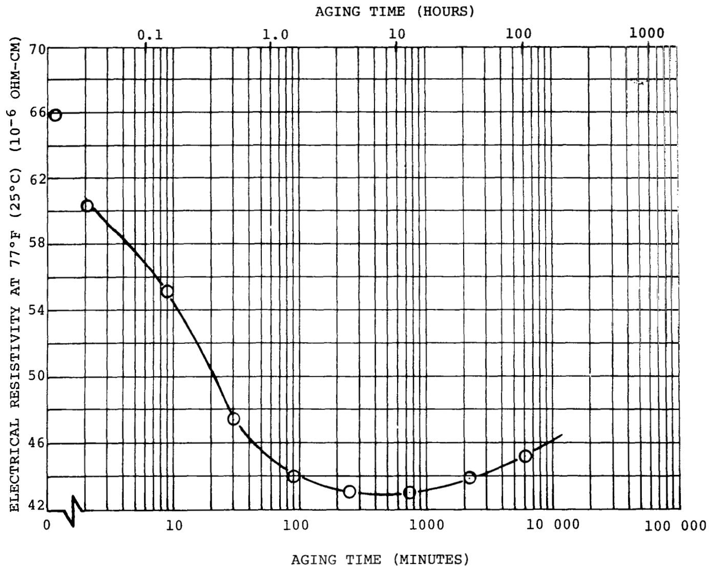
FIGURE II-24. Change in Room Temperature Electrical Resistivity of 15% Ni Maraging Steel (Fe-9Co-15Ni-5Mo-0.7Al-0.7Ti) During Isothermal Aging at 1112°F (600°C)
