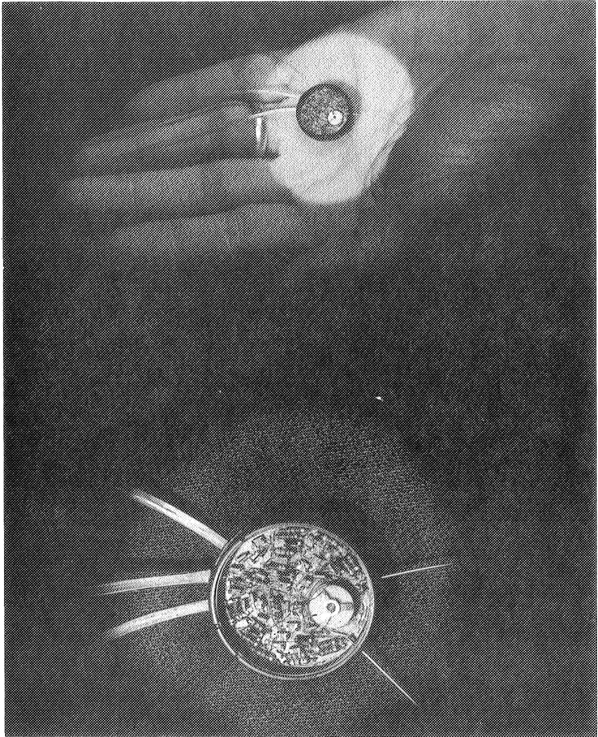
Fig. 1.0-4 Main Chassis Wired in Place, with Cell and Thermistor Leads
