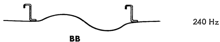
Figure 20 - Mode Shapes of a Nine Bay Configuration Specimen
