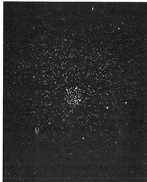
d. Image Obtained With Detector Adjusted for X-Rays From Silver
