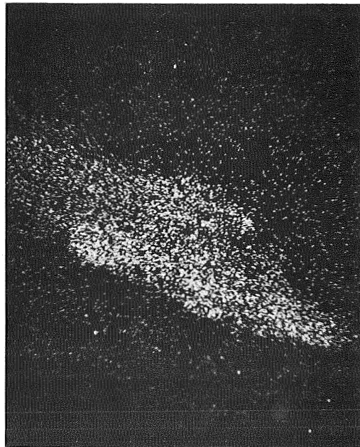
d. Image Produced by X-Rays From Silver
