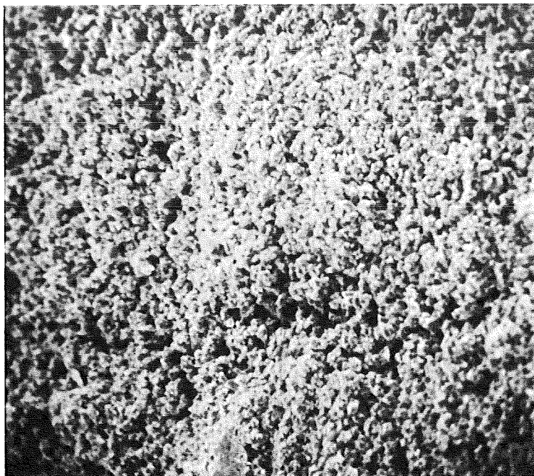
300 Magnification Silver Oxide Plate No. 83 As Received Flat Surface
