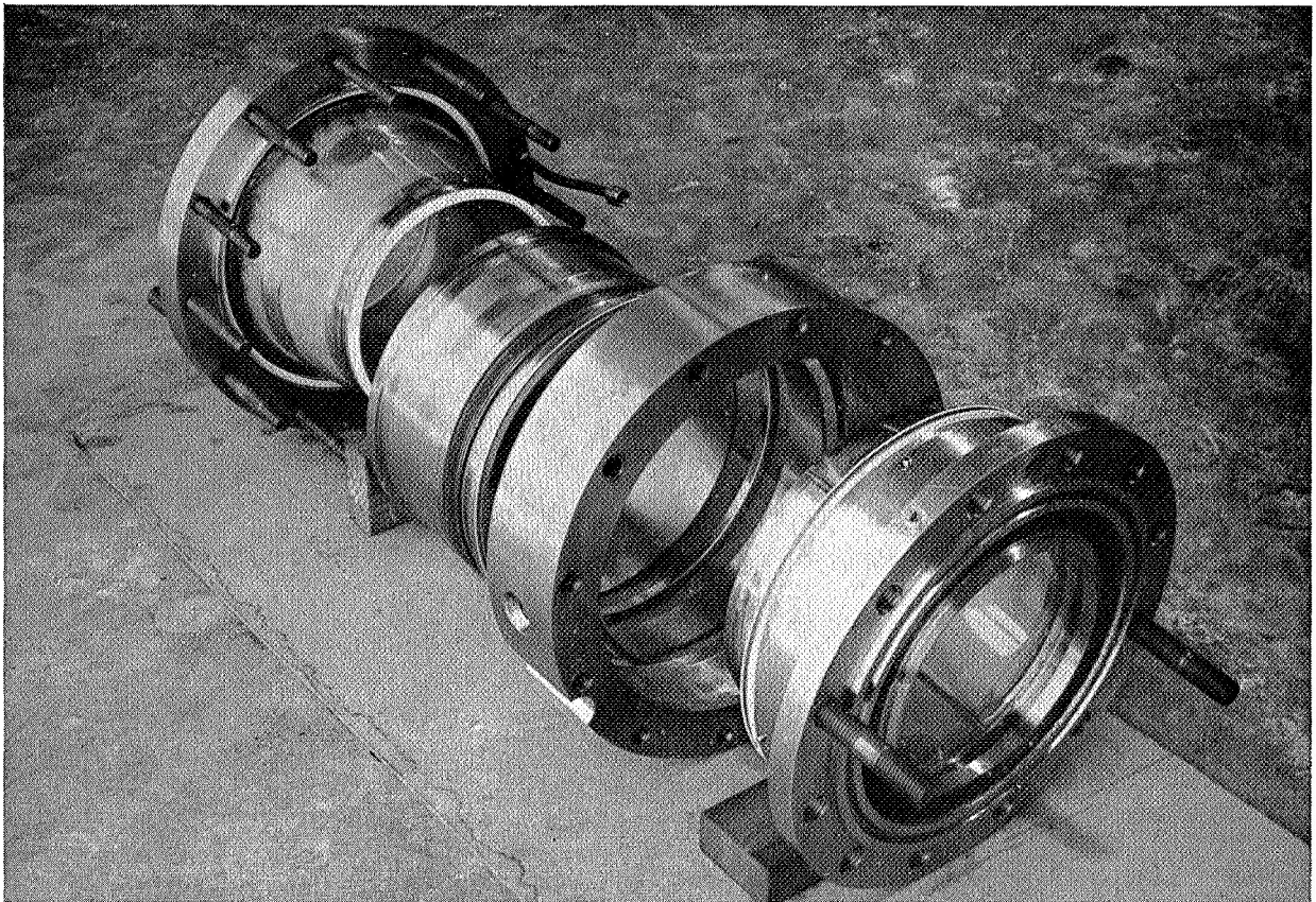
AMETEK/Straza 8-inch Rotary Joint — Disassembled Oblique Views from Both Ends
