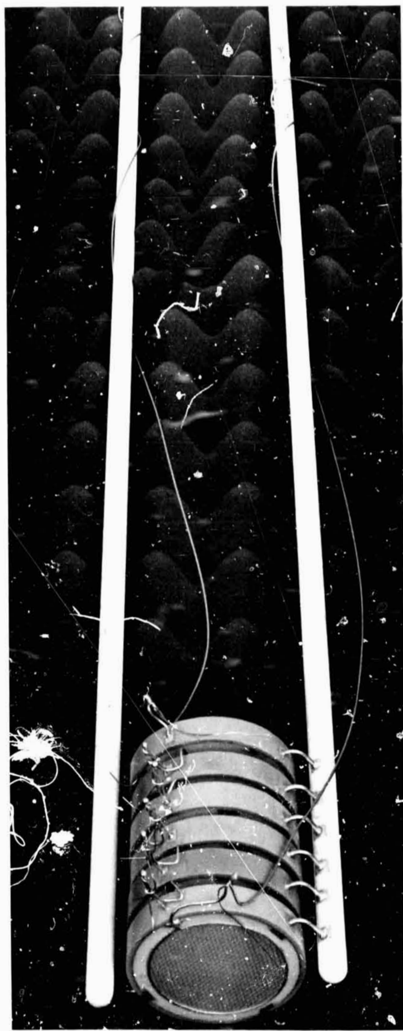
Fig. 6-4 Electrolyzer after Removal from Brazing Jig
