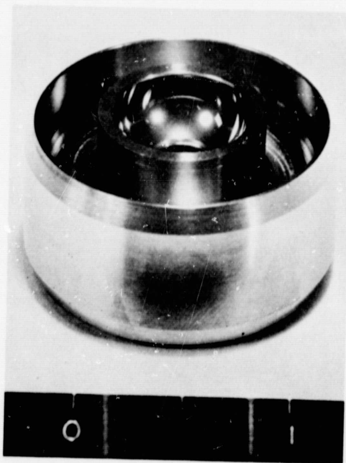
Fig. 13 Outer bearing in the beryllium wheel hub.
