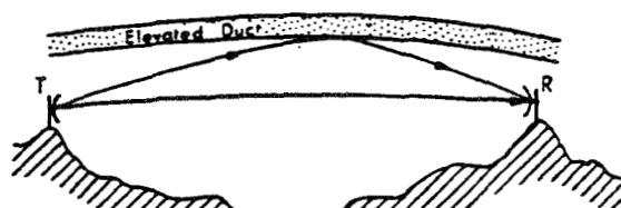
(b) Reflection by elevated duct
