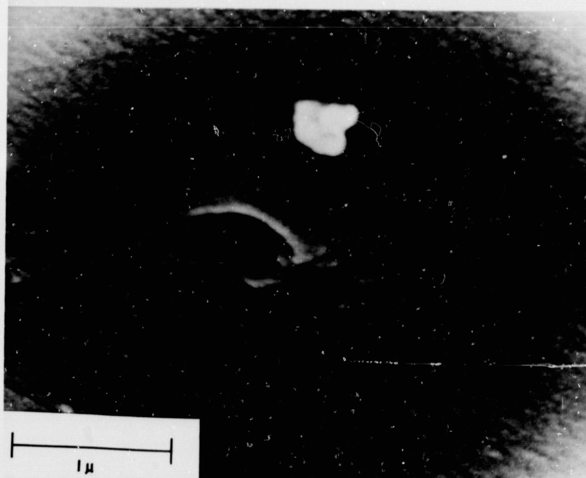
Fig.XII Small crater of probable impact origin, in a stainless steel sample.
