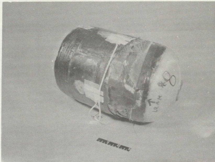
Figure 28. Post-burst View of Bottle No. 8 with Four-Ply Inverted Repair
