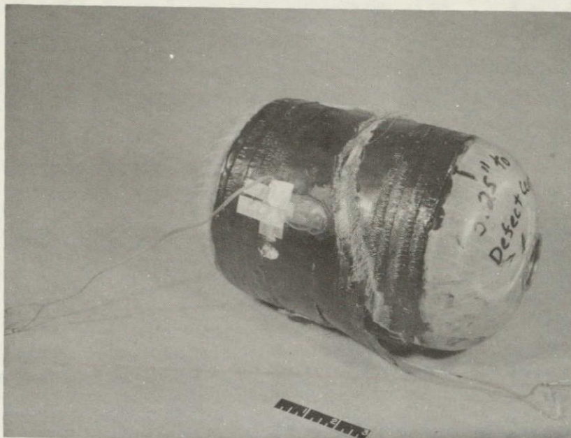
Figure 25. Post-burst View of Bottle No. 5 with Four-Ply Inverted Repair
