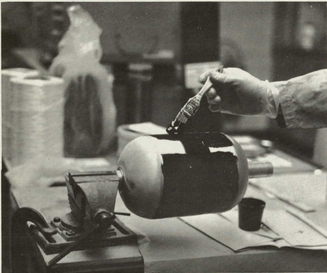
Figure 15. Adding Epon 946 Resin Coat to Repair Area
