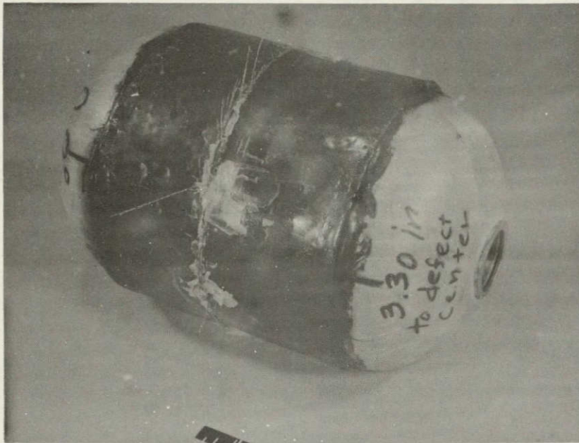
Figure 10. Bottle No. 3 - Post Test View of Three-Ply Tension Failure
