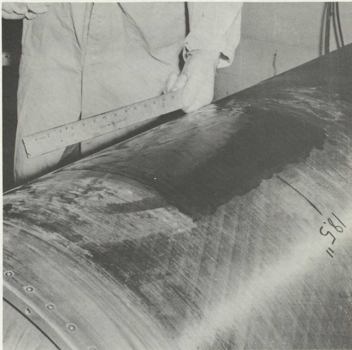
Figure 68. Patch Appearance After Application of Fourth Ply
