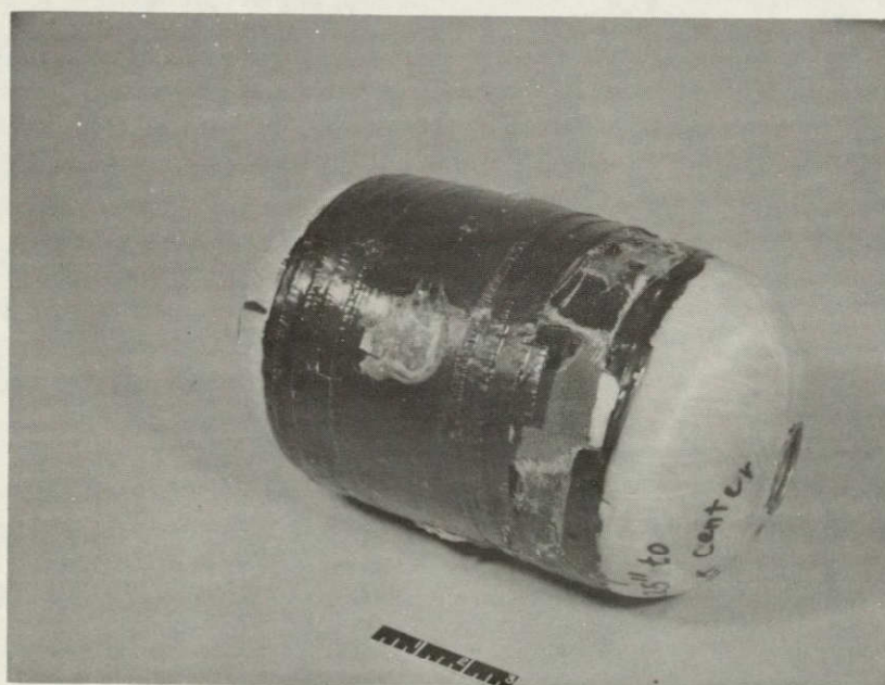
Figure 26. Post-burst View of Bottle No. 6 with Four-Ply Inverted Repair
