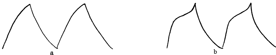
Fig. 4 -- a) normal electrode voltage response. b) distorted electrode voltage response.
