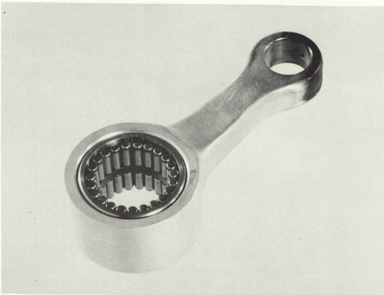
FIGURE 44. Connecting Rod after 90-hour Endurance Test in the SPU-3A Engine
