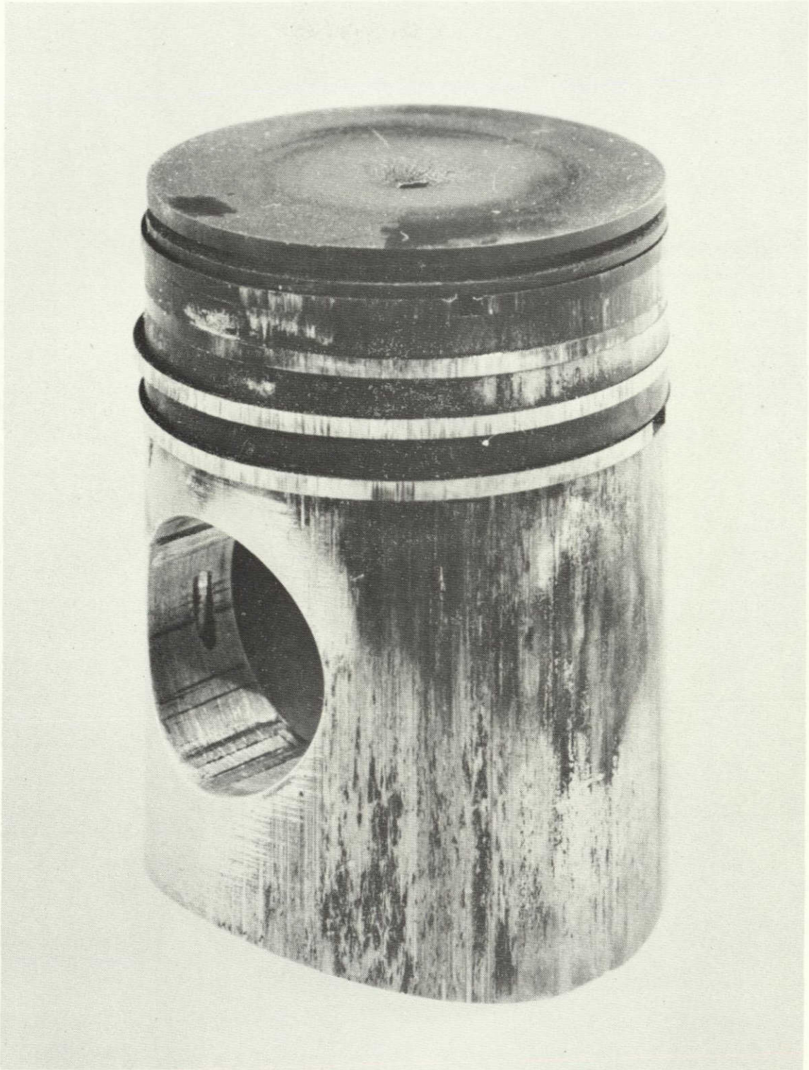
FIGURE 34. Modification 1 Piston Assembly after Test 5167/5
