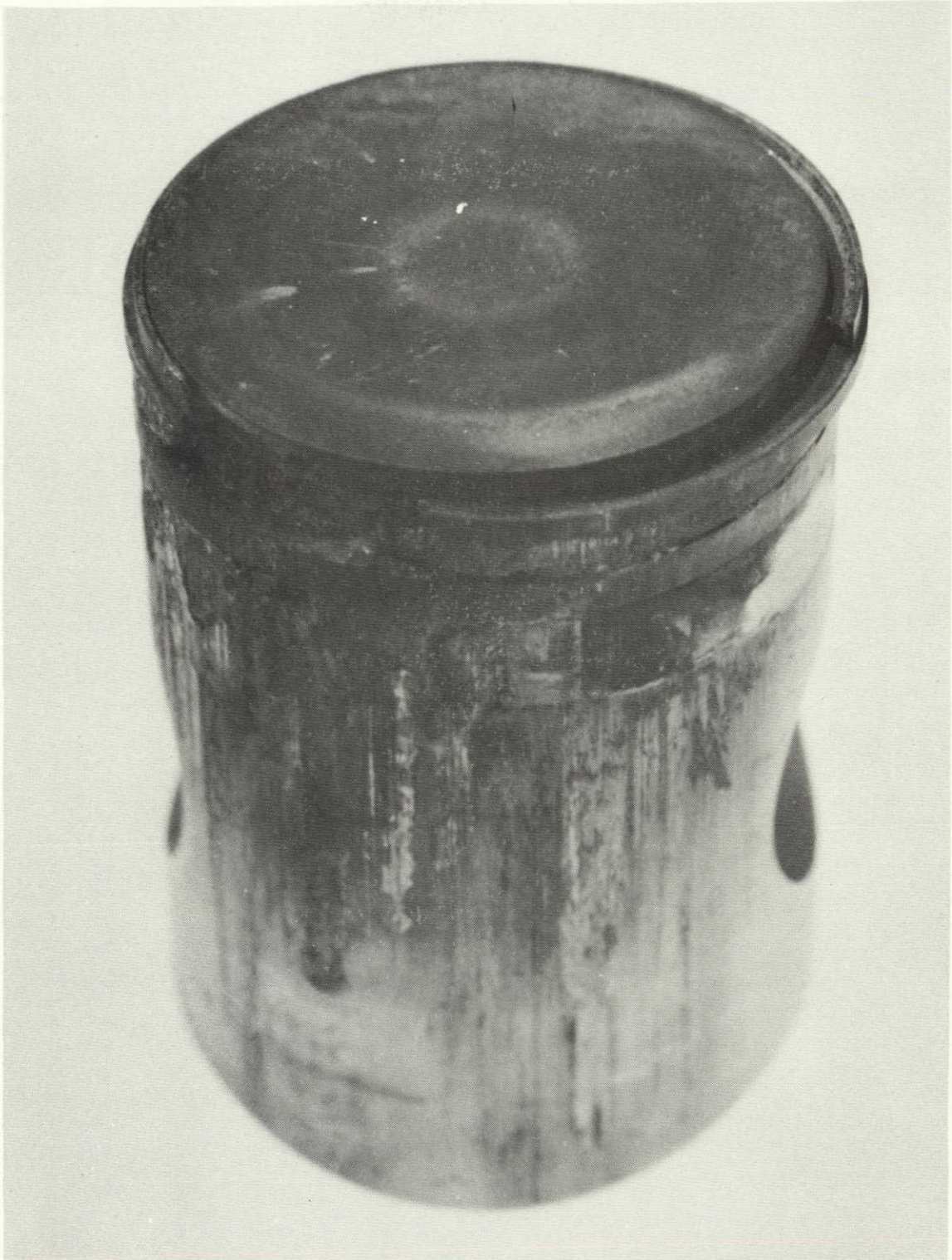
FIGURE 28. Configuration C Piston after Operation for 4.76 hours in the SPJ-2A-2 Engine
