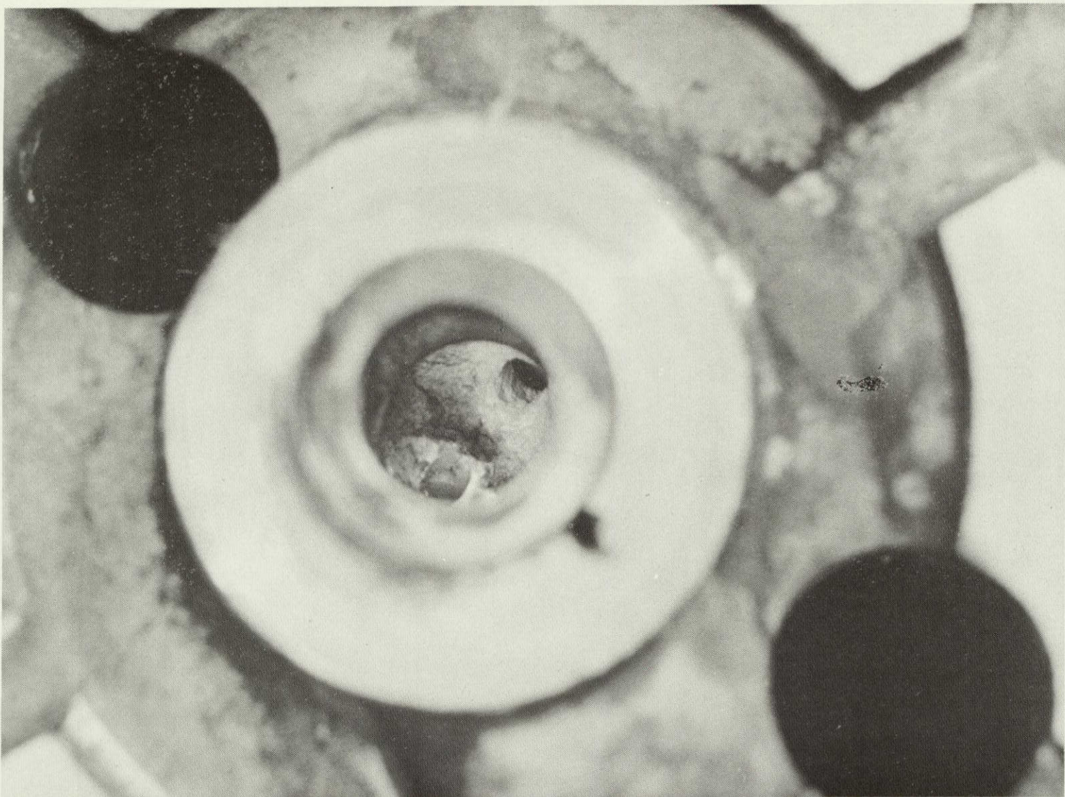
FIGURE 51. SPU-3 Cylinder Head Combustion Chamber after Test 5151-23
