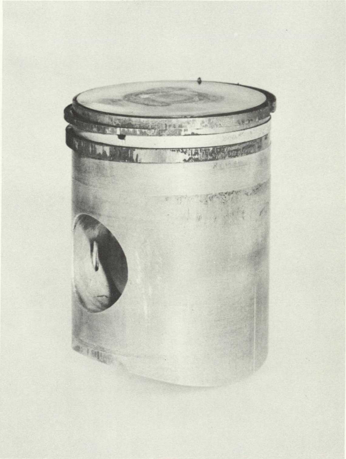
FIGURE 32. Piston Assembly with 440-C CRES Rings after 46-hour Endurance Test
