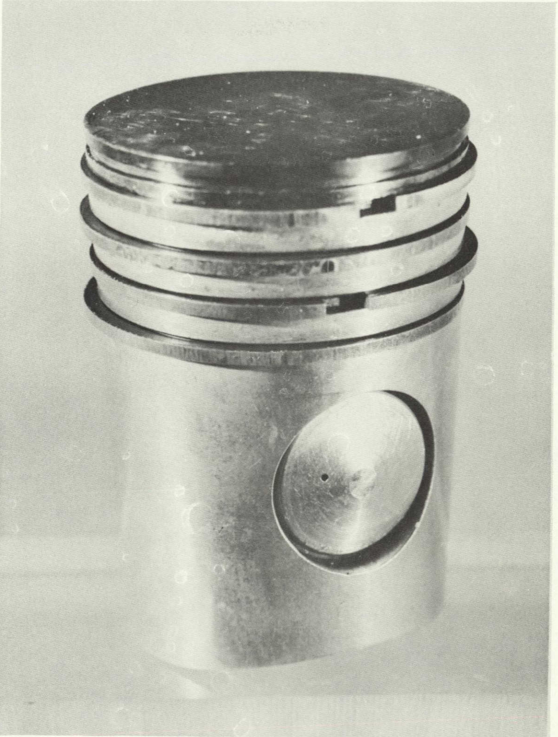
FIGURE 13. Modification 1 Piston Assembly Used in the SPU-3 Engine, After Test
