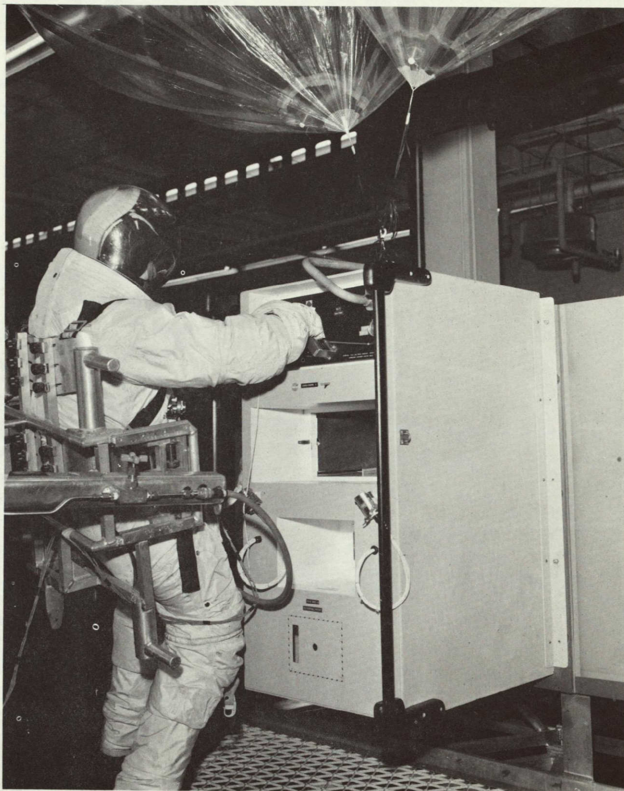
Figure 10-4. Removing Eva Box #1 Pressure Suit Zero-g Simulation With Eva Gloves
