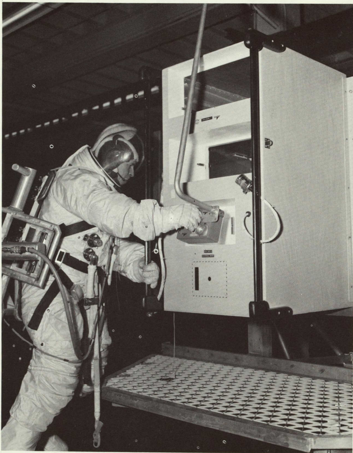
Figure 10-10. Removing EVA Box #3 Pressure Suit Zero-g Simulation
