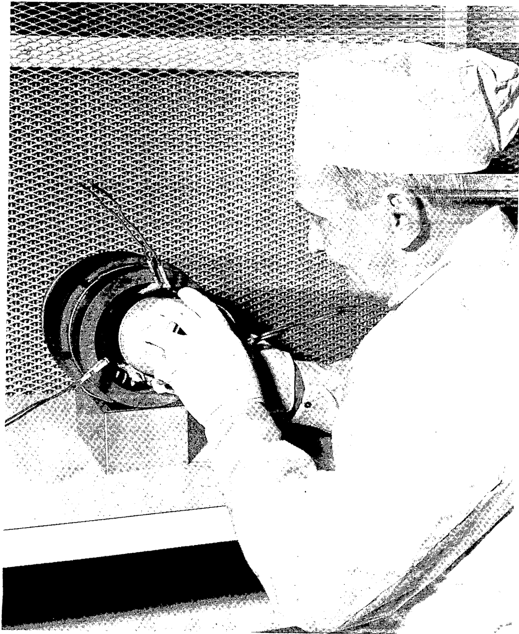
FIGURE II-25. Demonstration of the Bore Seal Capsule Fit Inside the Stator Cavity for the 1300° F 5000-Hour Endurance Test. In the Test Chamber the Stator Center Line is Vertical (leads up) and the Capsule sits on a pedestal.
