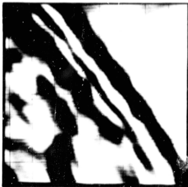
Fig. 8 - Section Pl-3D, Pahoehoe lava. Specimen current photograph showing concentrations of elements of high atomic number as light areas; concentrations of elements of low atomic number are shown as dark areas.
