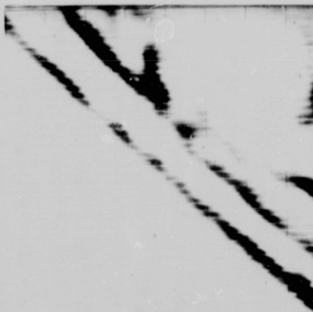
Fig. 13 - Section P1-3D. Pahoehoe lava. Specimen current photograph showing concentrations of elements of high atomic number as light areas and concentrations of elements of low atomic number as dark areas. Same area as figure 9 but specimen rotated 180^{\circ} .
