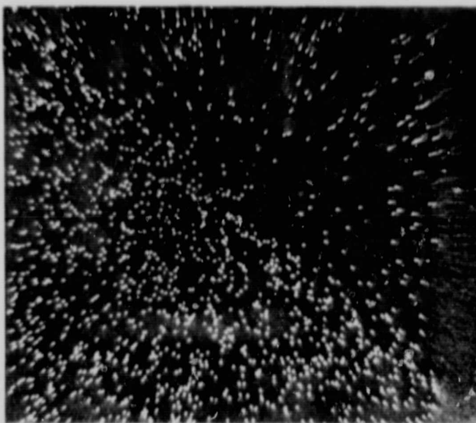
Fig. 12 - Section P1-3D. Pahoehoe lava. X-ray scanning photograph showing concentrations of Ti. Same area as figure 9 but specimen rotated 180^{\circ} .
