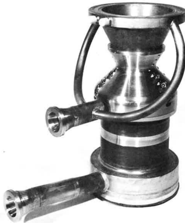
Fig. 24 30,000-lb high pressure LH 2 /LO 2 -thrust chamber
