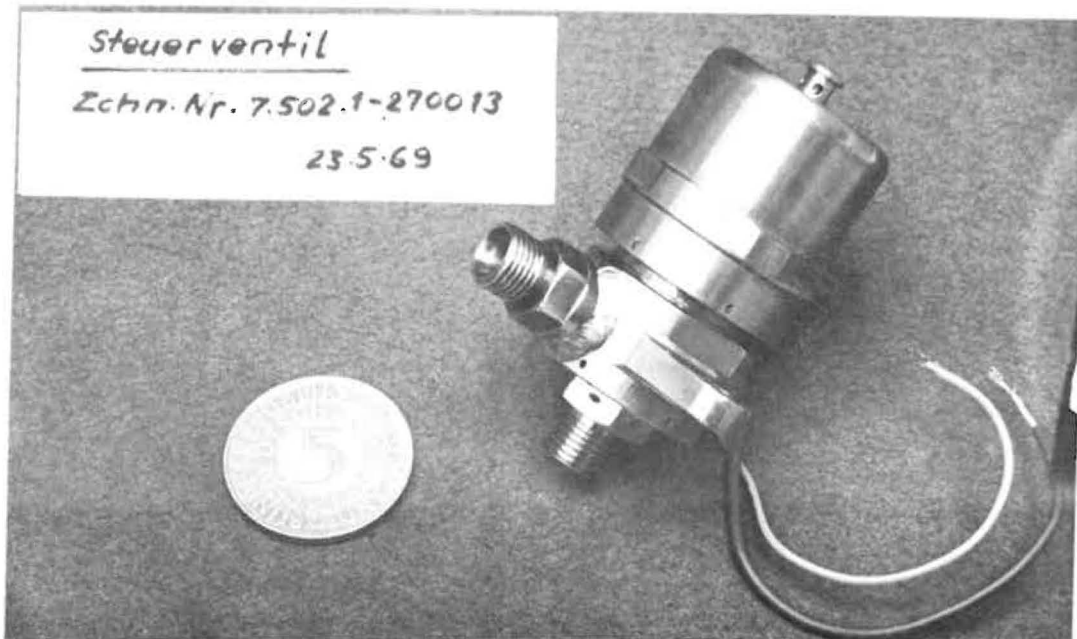
Fig. 14 Electromagnetic pilot valve for the LF 2 -main-shutoff valve
