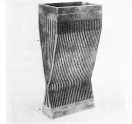
Ni, CAST CHANNEL WALL ELECTROFORM CLOSEOUT
