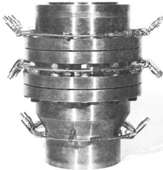
Fig. 4 Segmented heat sink 1,100-lb \text{H}_2/\text{F}_2 experimental engine for sea level testing, with thermocouples installed
