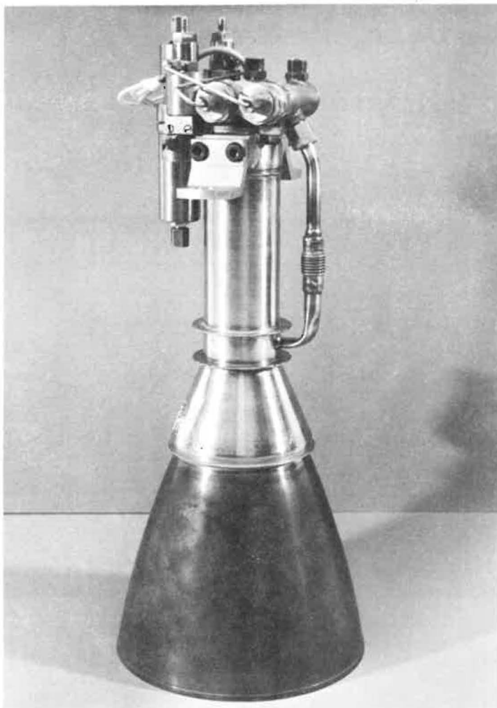
Fig. 16 Final version of the 66-lb \text{LH}_2/\text{LO}_2 -engine with its main propellant valves on top of the chamber and the igniter capsule left of the chamber
