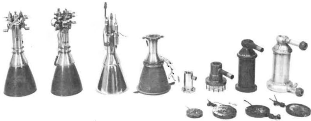
Fig. 15 Development history of the 66-lb \text{LH}_2/\text{LO}_2 -engine
