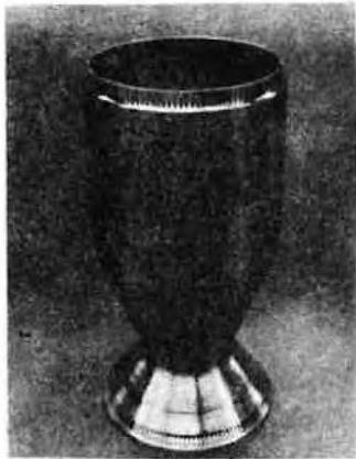
NICKEL, MILLED CHANNEL WALL ELECTROFORMED CLOSEOUT
