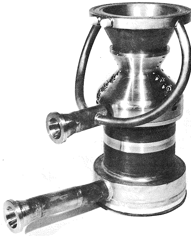
Fig. 24 30,000-lb high pressure LH 2 /LO 2 -thrust chamber
