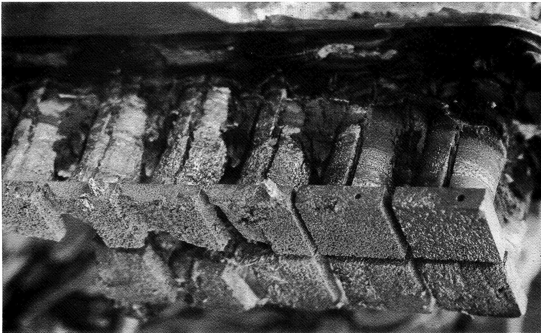
Figure 4. Damaged SiGe Stage
