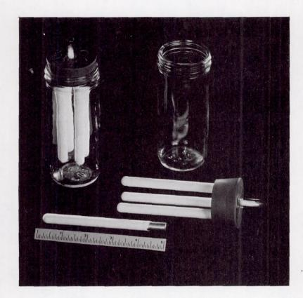
Figure 2. Specimens and Container Jar for Storage and High Humidity Study
