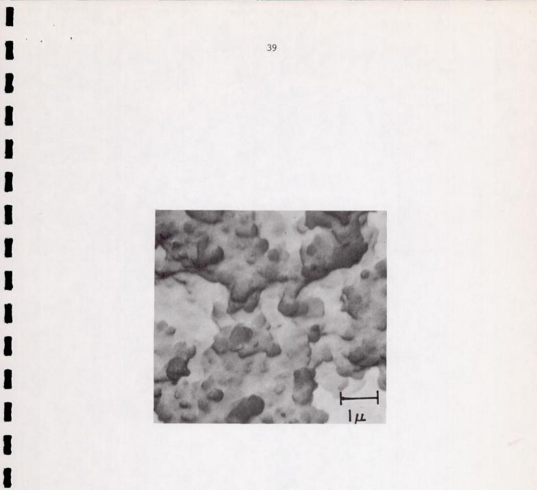
Figure 8. Control (Non-Exposed) Surface of Coating N-17 After Ultrasound Cleaning: SEM - 10,000X
