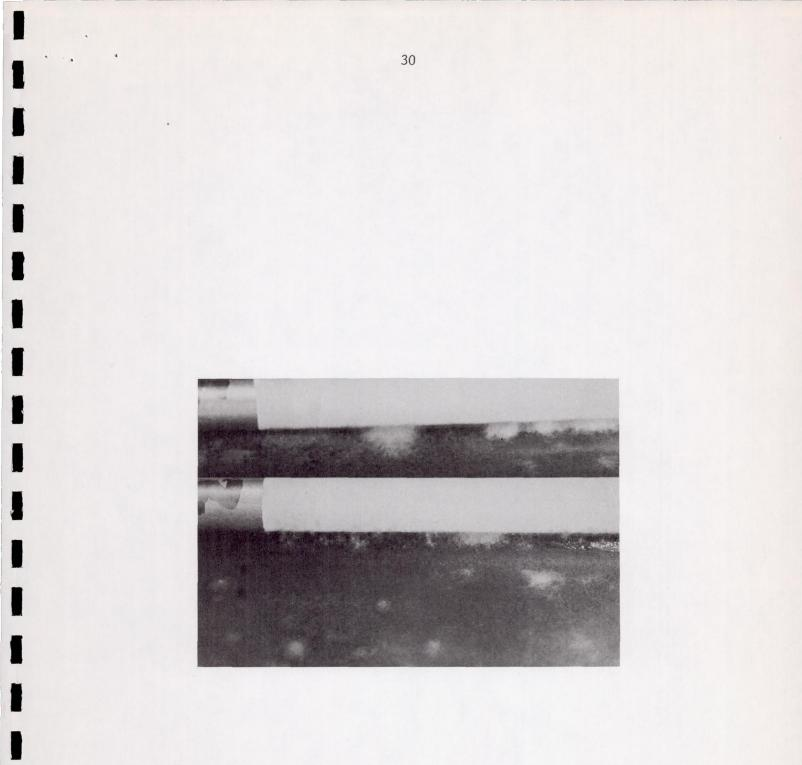
Figure 4. Typical Fungal Growth on Coating N-14 (Polyurethane) in Petri Plate Study on Mineral Salts Medium
