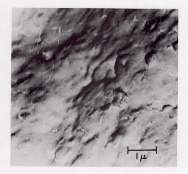
Figure 9. Surface of Coating N-17 After 4 Months of Soil Burial Exposure and Ultrasound Cleaning: SEM - 10,000X
