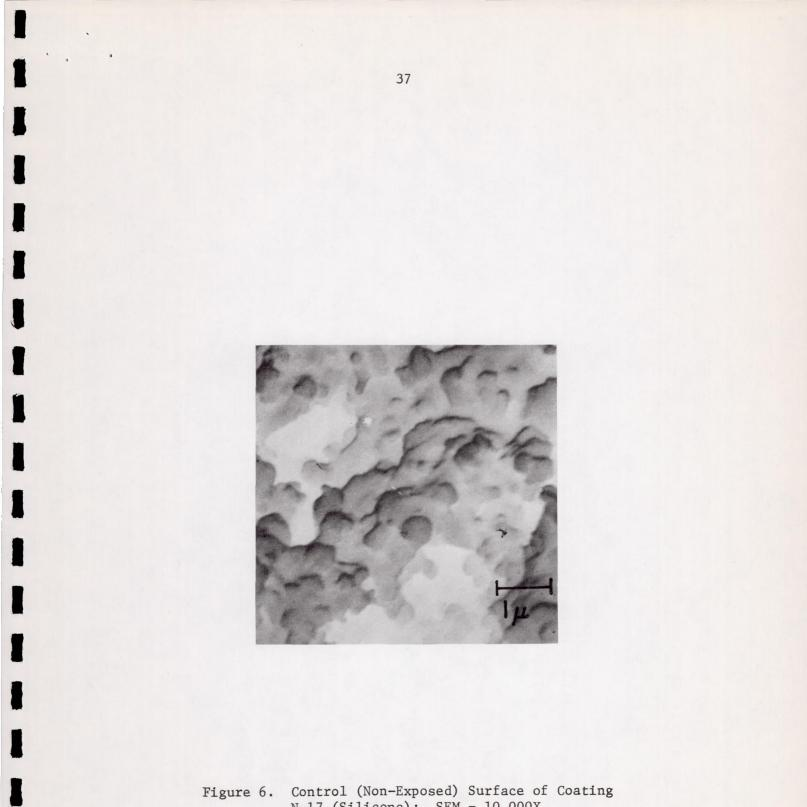
Figure 6. Control (Non-Exposed) Surface of Coating N-17 (Silicone): SEM - 10,000X
