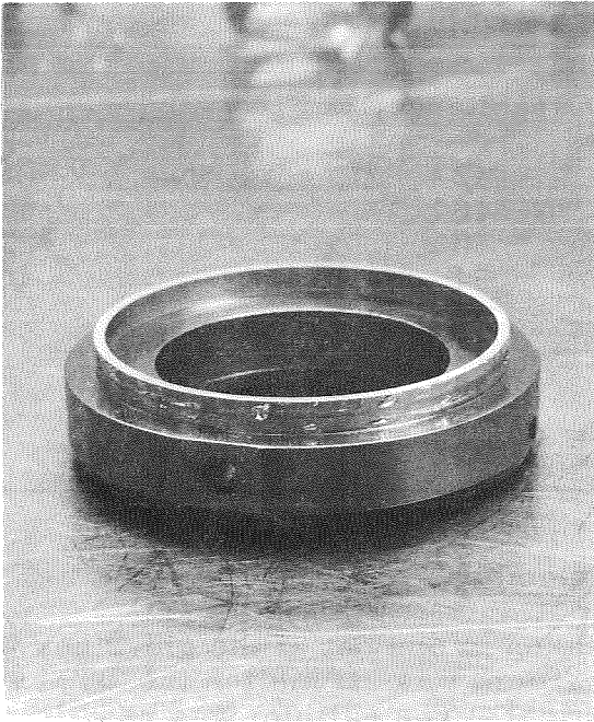
a) Inner ring after attempted fill. Circumferential track is from dial indicator used to check runout.
