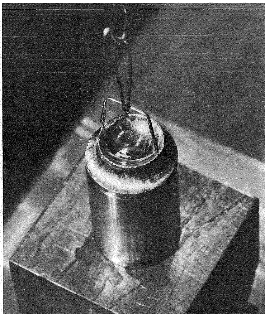
FIGURE 15. Measurement of Surface Tension by Ring Removal
