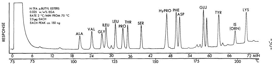
CONDITIONS: AEROGRAPH 2100; 2.5 µg EACH AMINO ACID DERIVATIZED; EACH PEAK REPRESENTS ca. 150 ng; SAMPLE VOLUME 80 µl; INITIAL TEMP. 75 °C; RATE 2 °C/MIN; 1.5m x4mm I.D. GLASS COLUMN; 0.325 w/w% EGA ON 80/100 MESH a.w. HEAT TREATED CHROMOSORB G; 70 ml/MIN N2
