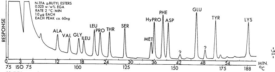
CONDITIONS: AEROGRAPH 2100; SAMPLE: 1.0  $\mu$ g EACH AMINO ACID IN 80  $\mu$ l, (5 $\mu$ l) INJECTED, 60ng EACH, COLUMN:1.5 m  $\times$  4 mmlD., GLASS WITH 0.325 w w<sup>2</sup>c EGA ON 80/100 MESH a.w. HEAT TREATED CHROMOSORB G, INITIAL TEMP. 75 °C, PROGRAM AT 2 °C MIN TO 195 °C, SENS. 1 x 2. N<sub>2</sub> flow 70ml MIN.
