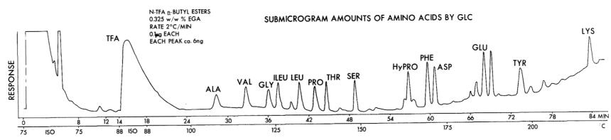
CONDITIONS: AEROGRAPH 2100; SAMPLE: 0. ومياة EACH AMINO ACID IN 80 ألمو; 6ng EACH(ألبوك) INJECTED; COLUMN: 1.5m×4mmiD, GLASS WITH 0.325 w/w% EGA ON 80/100 MESH a.w. HEAT TREATED CHROMOSORB G; INITIAL TEMP. 75°C, PROGRAM AT 2°C/MIN TO 195°C; SENS. 1×2.
