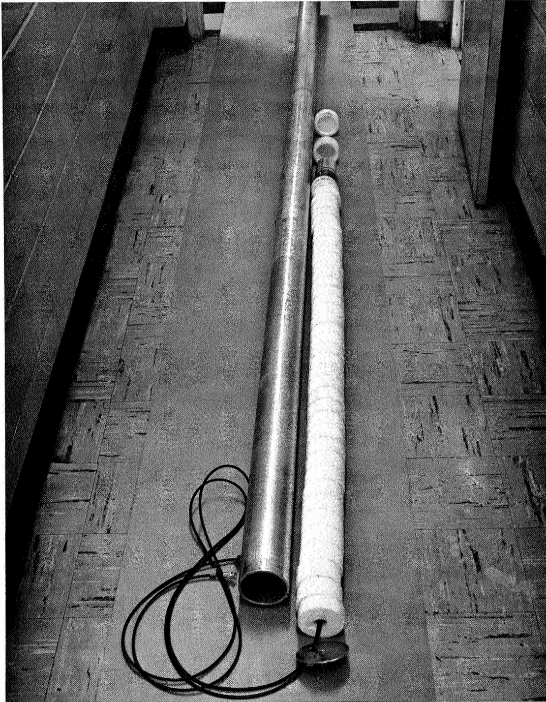
Figure 5-1. A Partially Disassembled Traverse Tube Showing One of RSG-8A Chambers and the Method of Assembly
