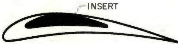
(C) VANE 3. INTERNAL INSULATING INSERT
