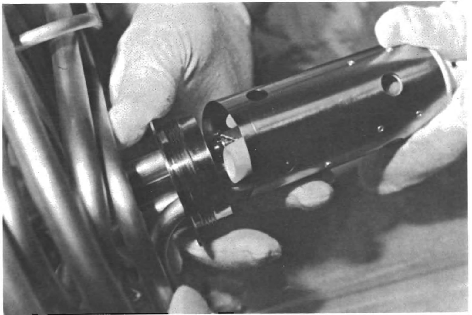
Figure C-4.23 - Final mating of quantity probe and tank adapter.
