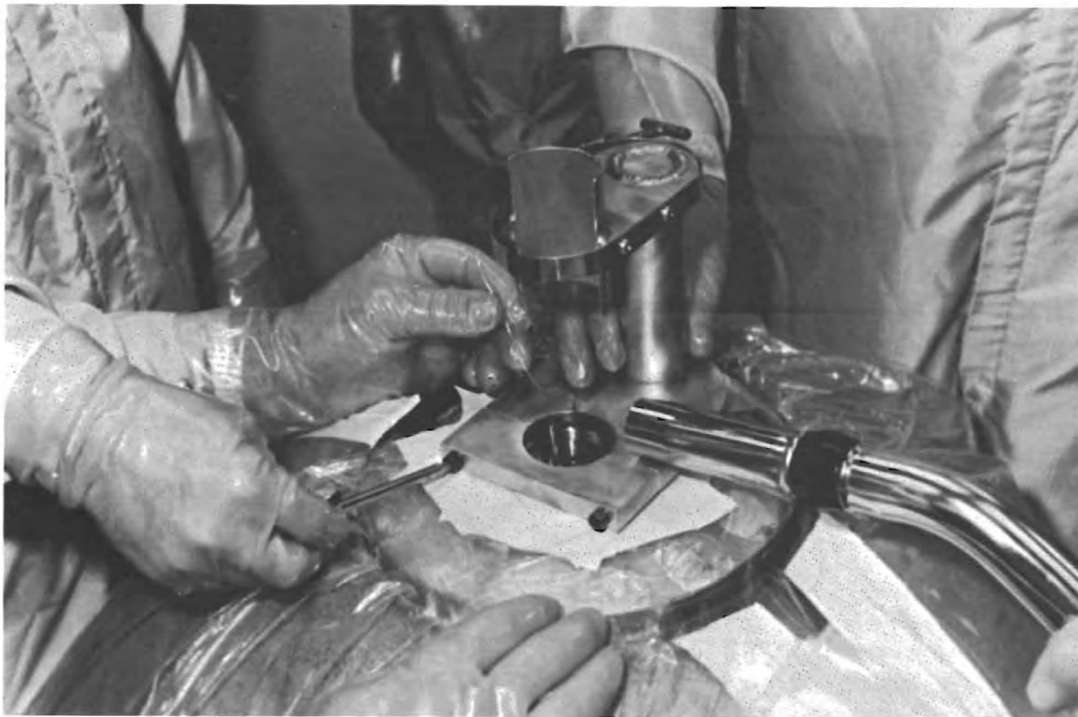
Figure C4-38.- Lowering wires into tank with fixture to hold quantity probe installed.
