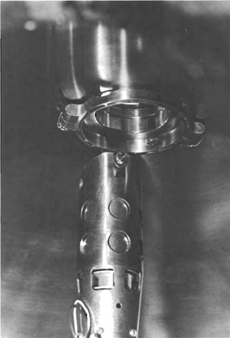
Figure C4-36.- View inside tank showing heater probe upper retaining bolt.
