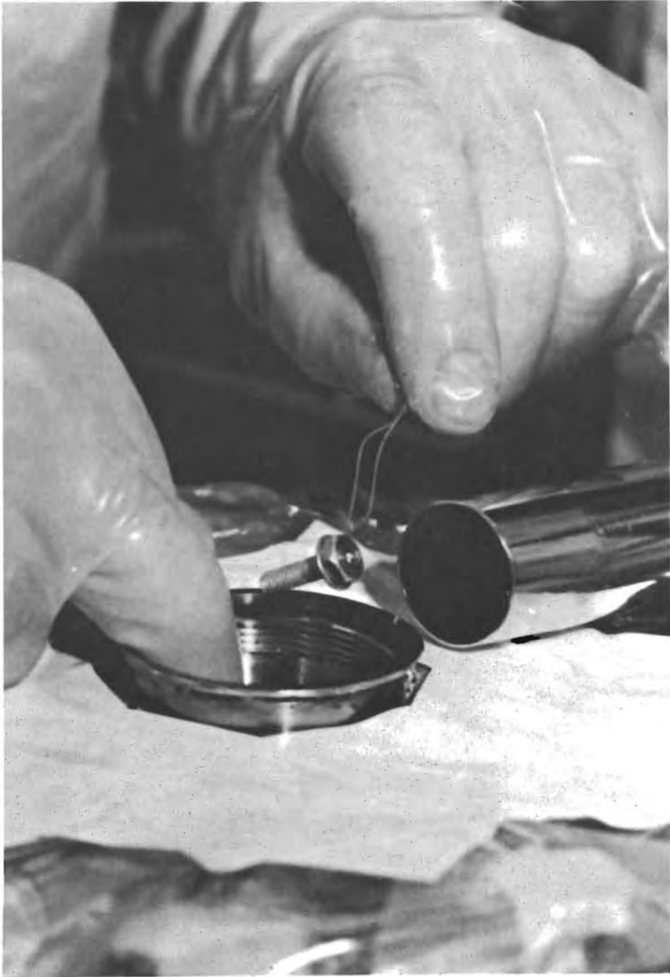
Figure C4-35.- Wire loop used to install heater probe retaining bolt.
