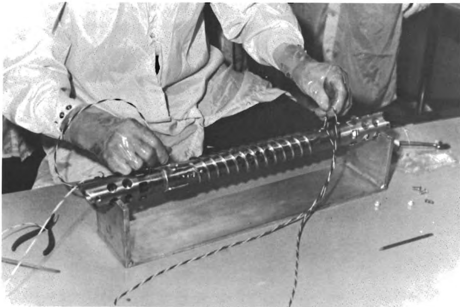
Figure C4-12.- Installing lower motor lead wires in heater conduit.
