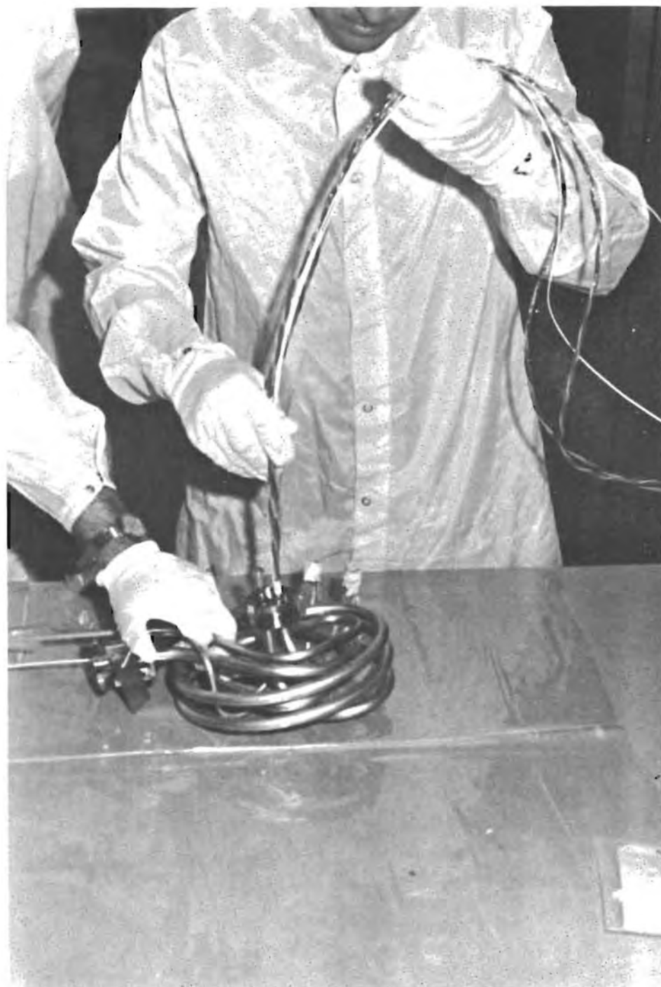
Figure C4-17.- Feeding quantity probe wires into upper coil assembly.
