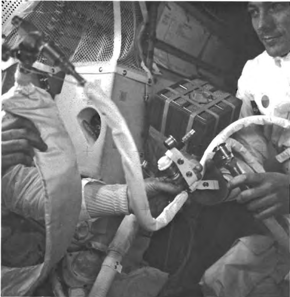
Figure B6-7.- View of CM LiOH cannister modification as installed in the LM.
