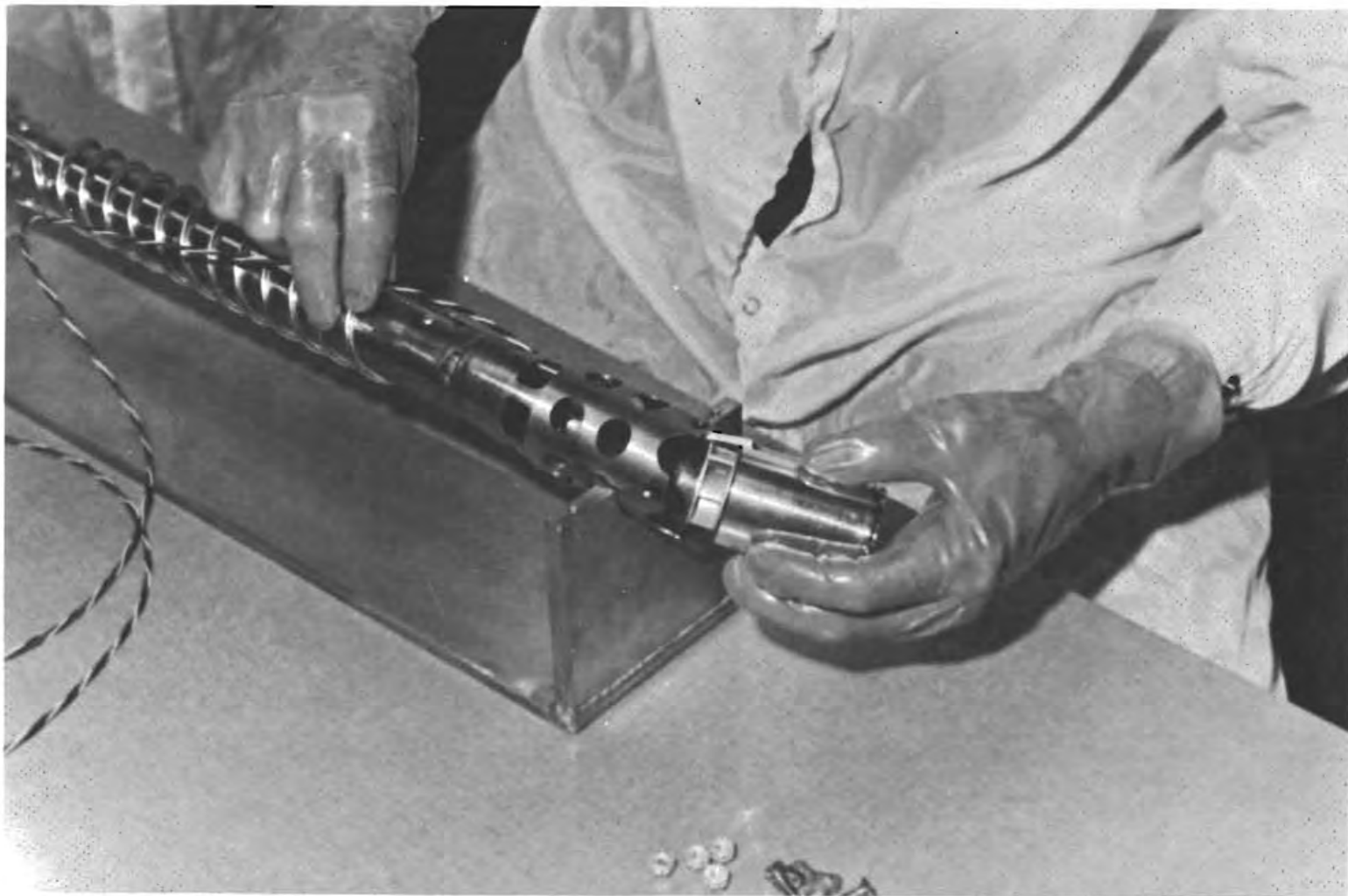
Figure C4-9.- Installing lower fan motor.
