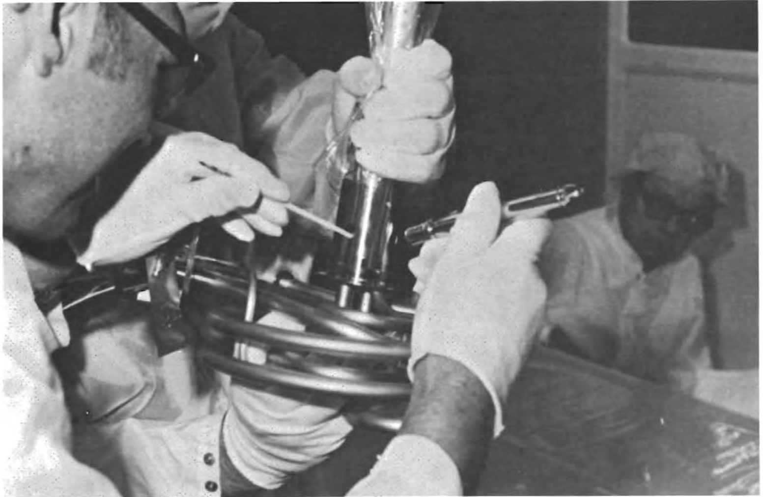
Figure C4-24.- Probing to assure that fill tube parts are in proper position.
