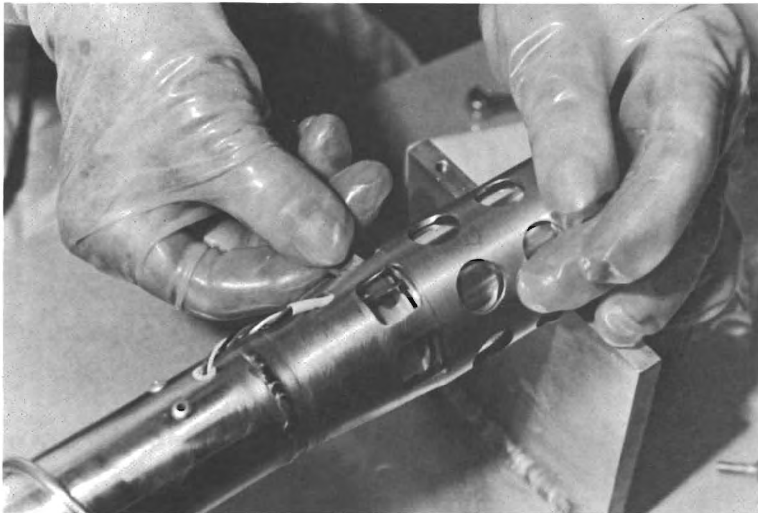
Figure C4-13.- Inserted copper band to retain motor wires.
