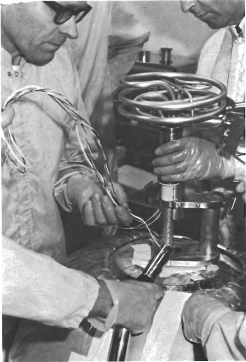
Figure C4-39.- Quantity probe being installed in fixture and heater probe wires being pulled from the tank.
