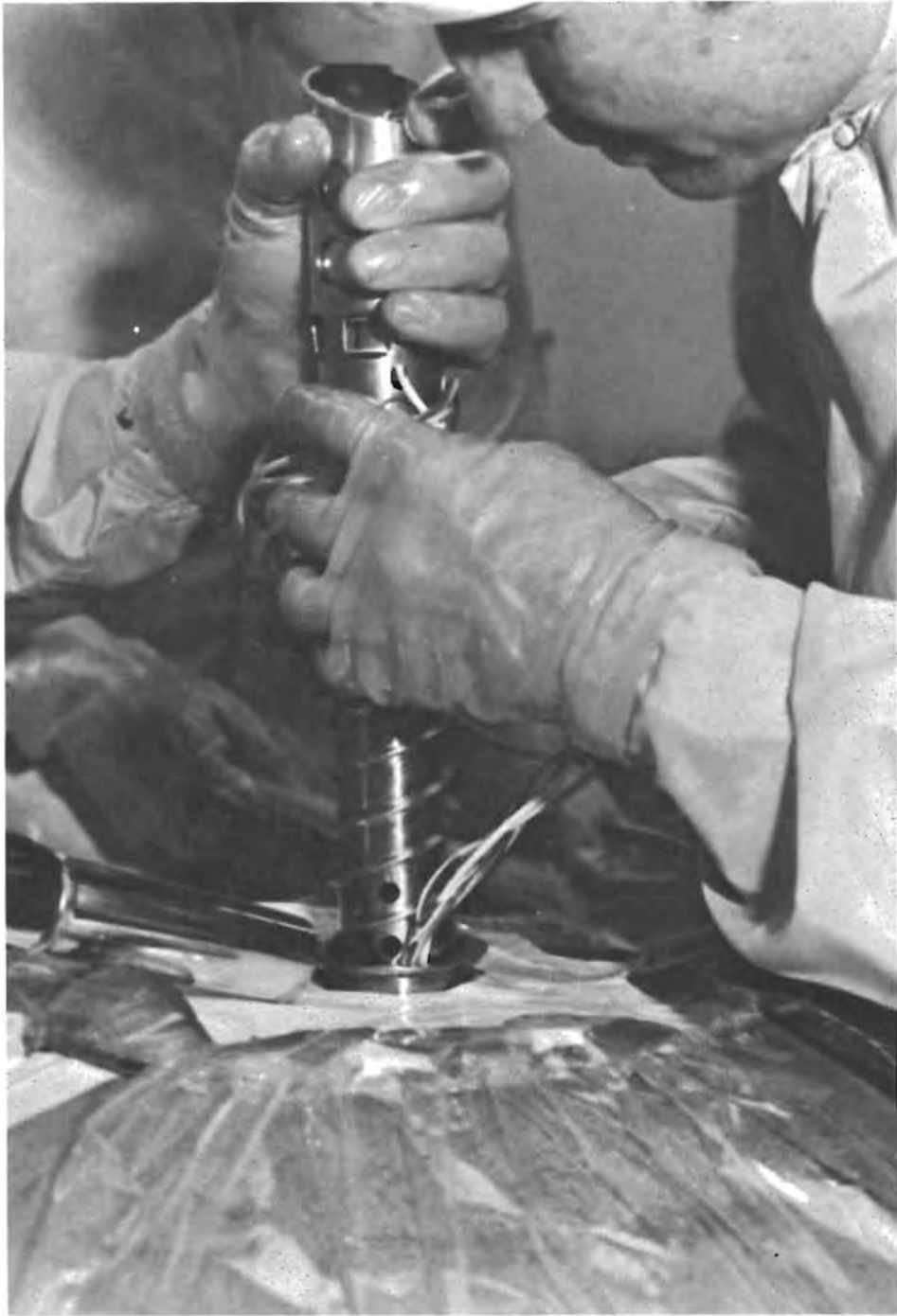
Figure C4-32.- Feeding wires into tank beside heater probe.
