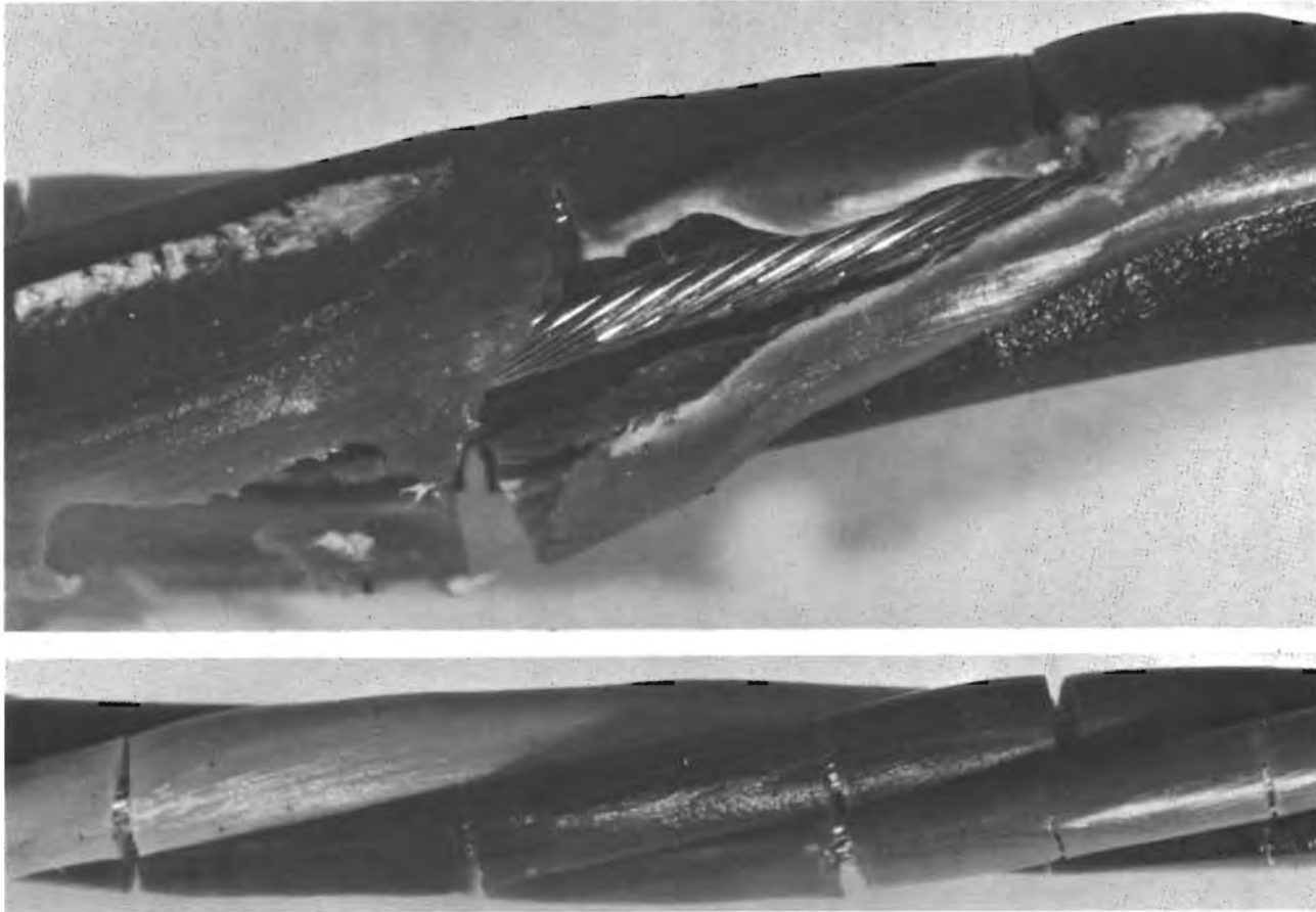
Figure C4-68.- Wire damage from heater tube assembly temperature test.
