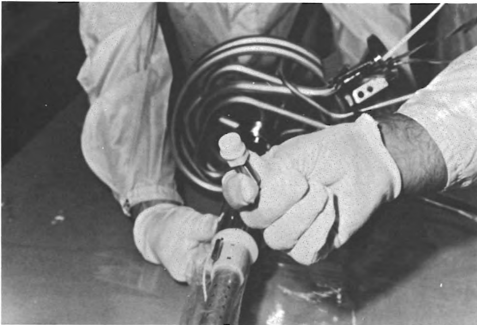
Figure C4-21.- Installing fill tube connecting parts.
