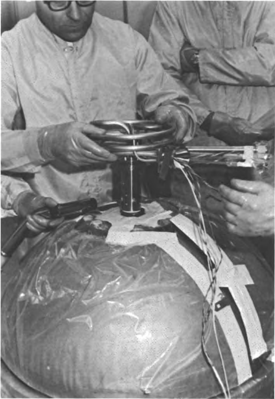
Figure C4-44.- Lowering quantity probe assembly into tank.
