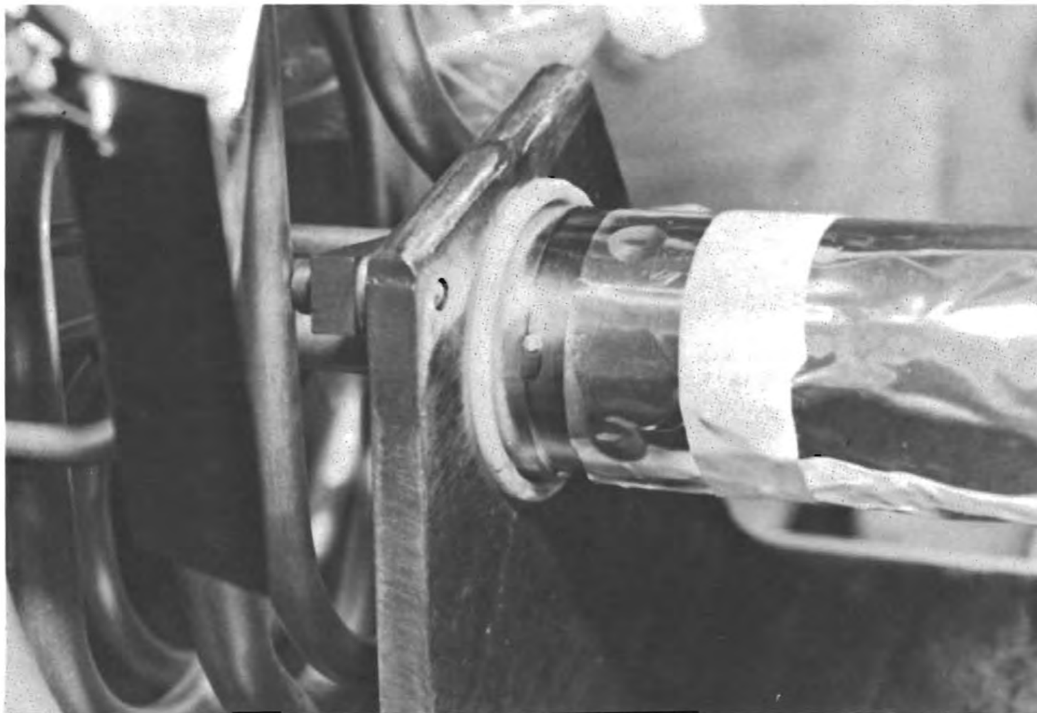
Figure C4-29.- The completed quantity probe to coil assembly welds.
