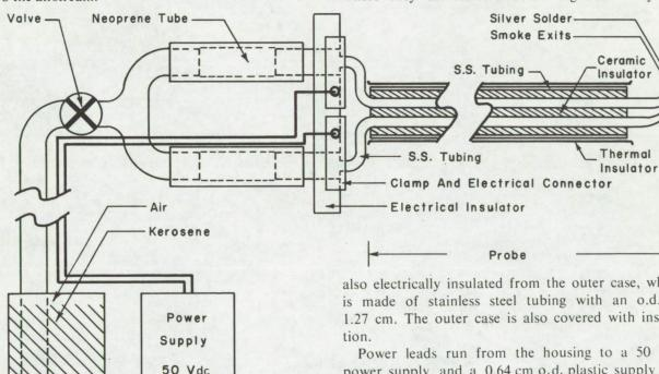
The device incorporates a smoke generation concept used in European devices: Kerosene is vaporized by electrically heating the tubes that carry the kerosene down the probe. Smoke is emitted from orifices at one end of the 18-cm-long probe. At the other end, a 2.54-cm-long housing (5.08 cm in diameter) encloses the kerosene and electrical connections, and serves as a handle. A kerosene flow adjust valve is attached to the housing.
