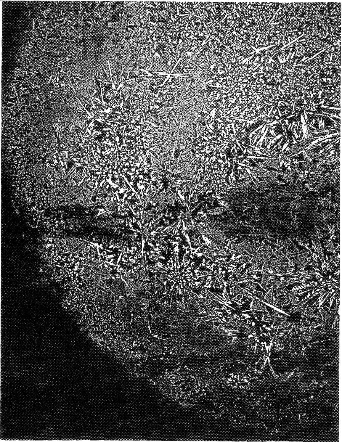
FIGURE 3. MOSAIC PHOTOMICROGRAPH SHOWING STRUCTURE OF A DROP CAST BALL OF STAR "J" STELLITE (Mag \times 62)
