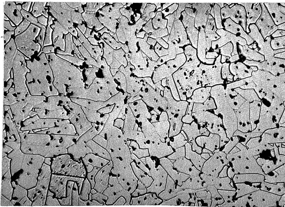
Figure 5. Etched Structure of SiC with 3 w/o \text{Al}_2\text{O}_3 and 1 w/o C. Billet 1237, Density 3.08 gm/cc, Grain Size 8 \mu .
