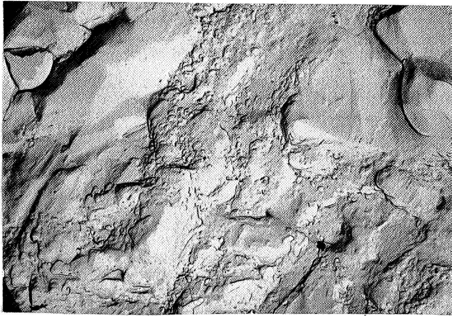
Figure 31. Fractograph of Si 3 N 4 Billet 1251 Broken at 2000°F (1366°K). Density 3.19 gm/cc, Grain Size .2 μ - Small, 2.5 μ Large.
