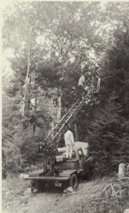
Figure 7-1.- Photograph showing method of obtaining reflectance data in a downward-looking orientation.
