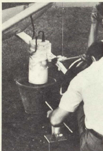
Figure 16-11.- Cross-calibration of radiation sensors. A basic calibrating device, the Leslie Cube is shown being applied to the ground PRT-5 thermometer (upper), a water bucket being used in calibration of the Barnes plane PRT-5 (lower left), and cross calibration of these devices to the RS-14 scanner of the NASA aircraft (lower right).
