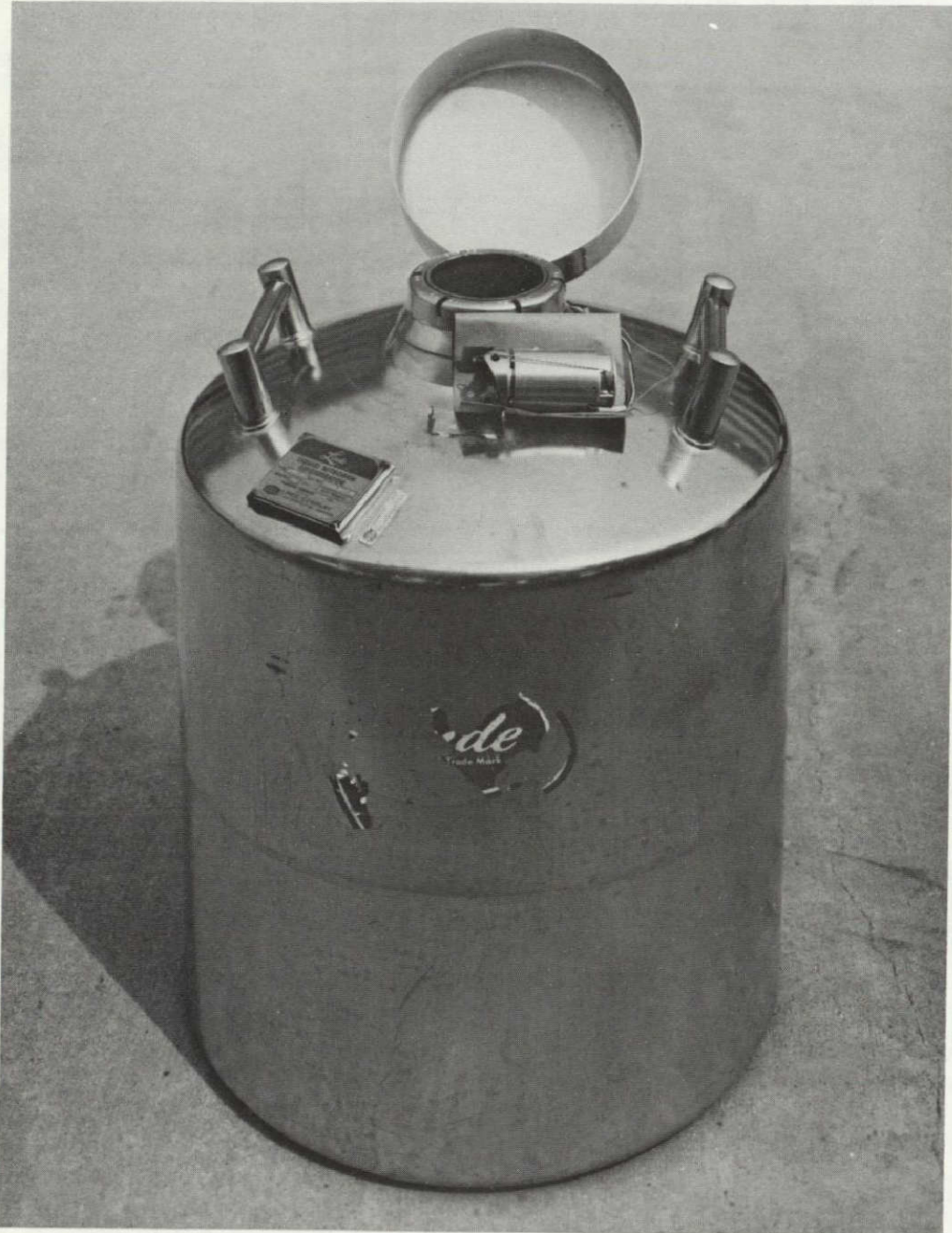
Figure B.19-2.- Destratification locked rotor investigation (motor shown with safety wire lock).
