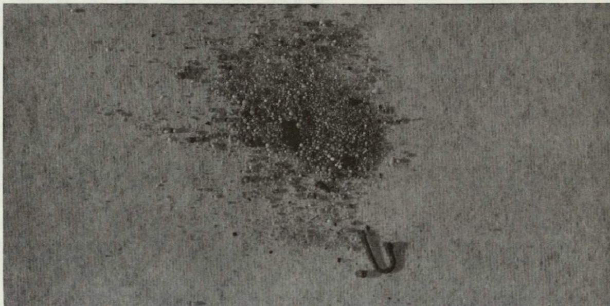
Figure B.14-7.- Post-test residue from aluminum ignition and complete combustion.
