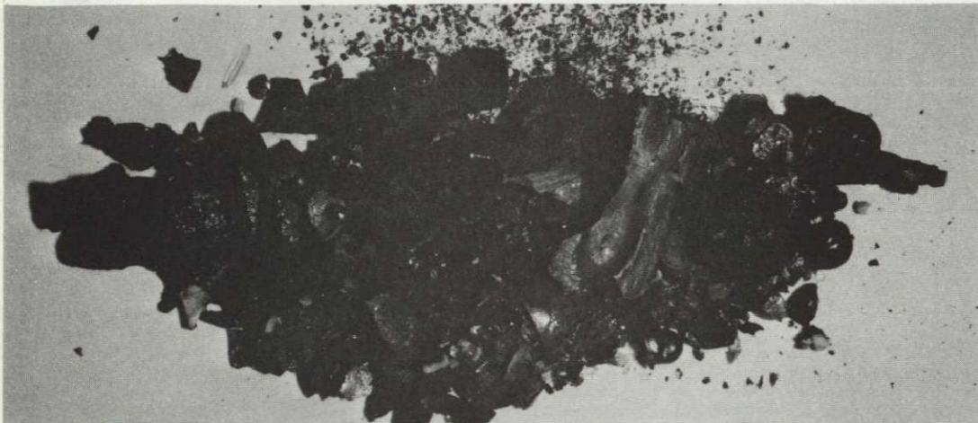
Figure B.14-10.- Post-test residue from Inconel X750 with wire bundle ignition.
