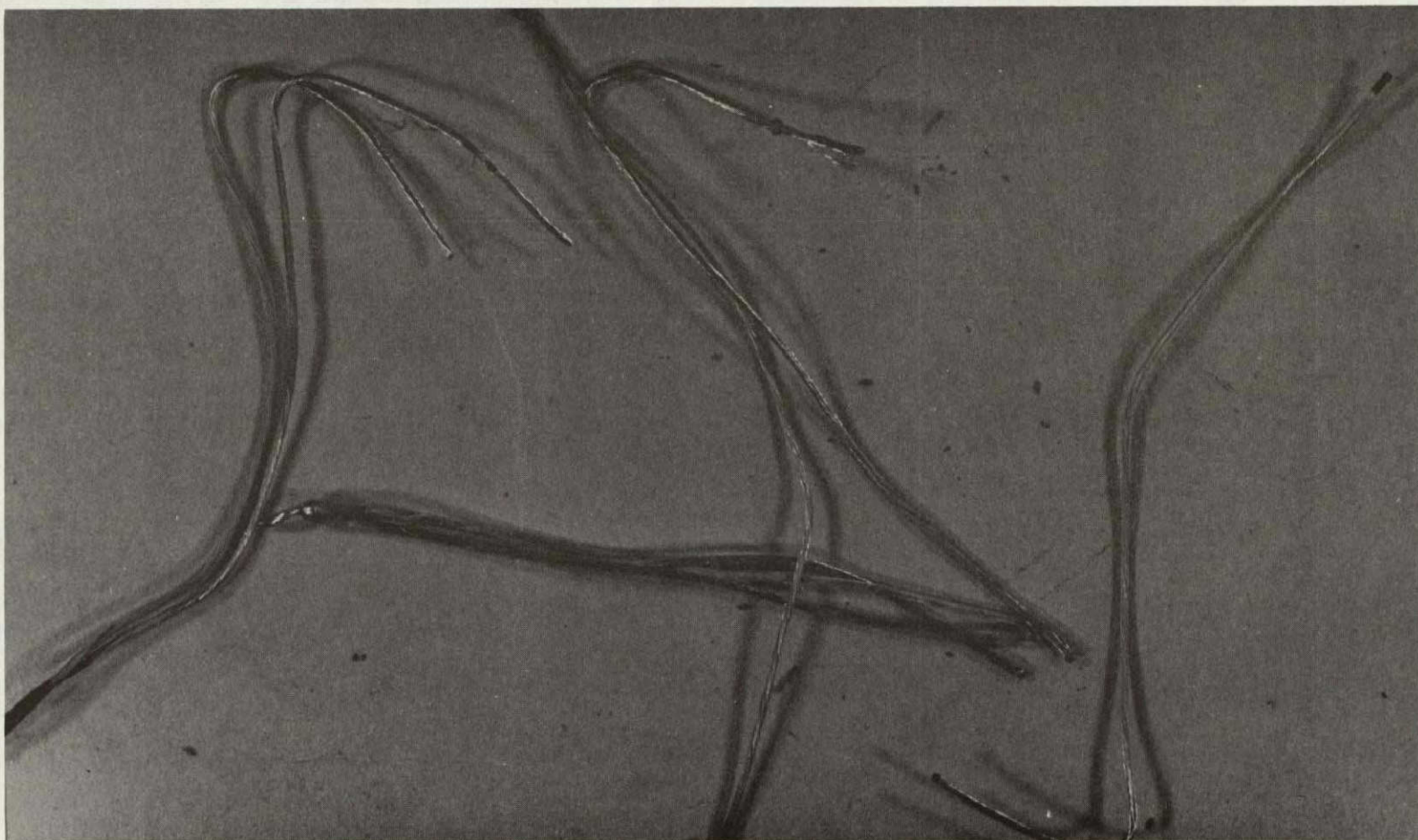
Figure B.35-7.- Four conductor wire in white tubing.
