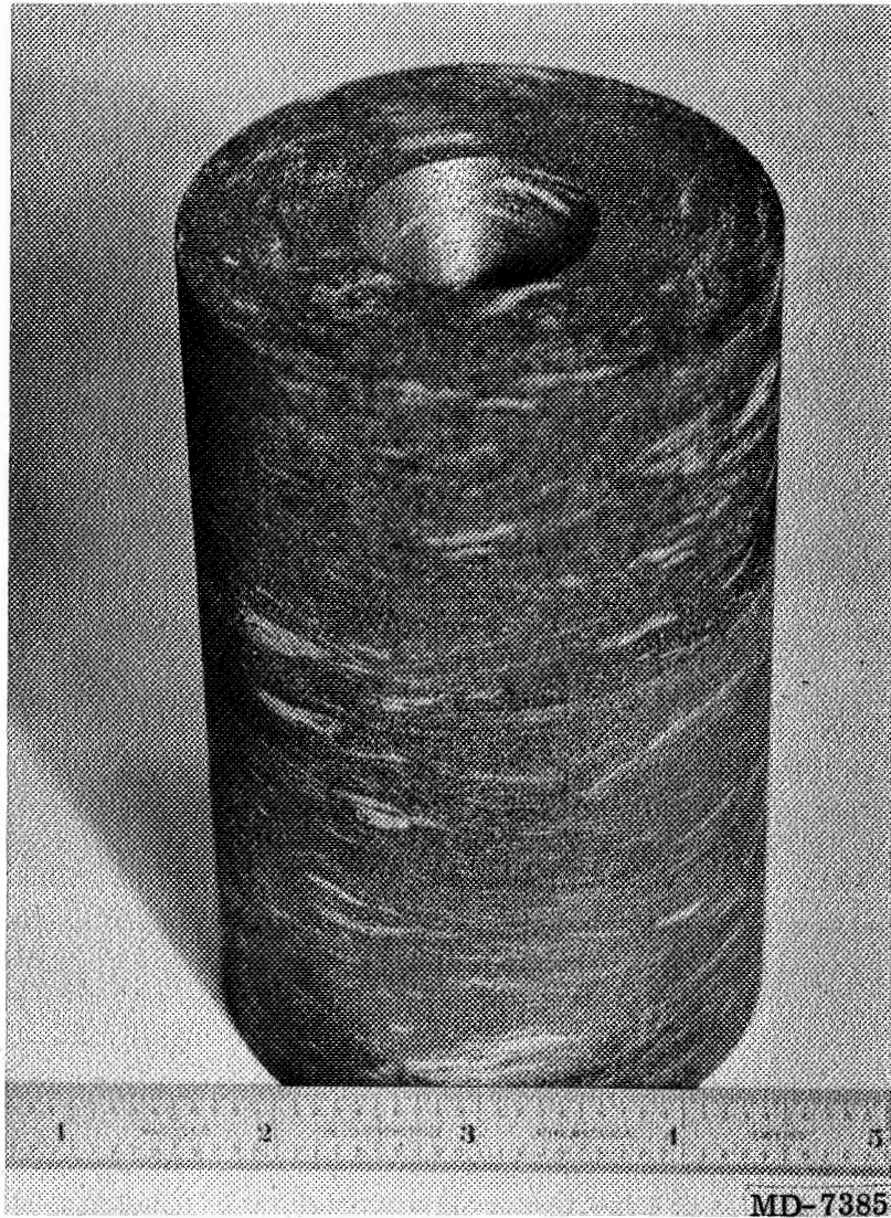
Figure 58. - Machined TU-379 Nozzle Assembly Showing Banding Effect
